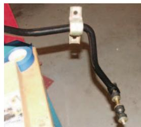
**Photo 4:** To locate the front anti-sway bar front to rear on the frame, the end links for the anti-sway bar must be installed on the bar.
