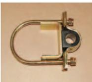
**Photo 13:** The rear anti-sway bar bolts to the rear end housing using a U-bolt and nuts, C-channel, urethane bushings and a U-clip. The rear anti-sway bar can be used on a stock rear end as well as a 10 or 12 bolt GM rear end or a Ford 9" with 3-1/8" axle tubes.
