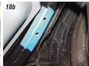
**Photos 18a & 18b:** With the frame marked, drill two 7/16" holes. The 7/16" holes will allow the 3/8" U-bolts to rotate into place.
