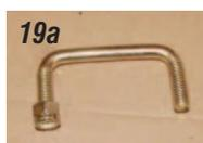
**Photos 19a, 19b & 19c:** Before installing the U-bolts in the frame, install one of the lock nuts on one end of the U-bolt. This will keep you from losing the U-bolt up in the frame.
