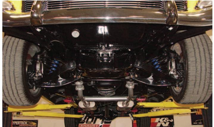
**Photo 1:** The front anti-sway bar mounts to the bottom of the frame rails just in front of the engine crossmember.
