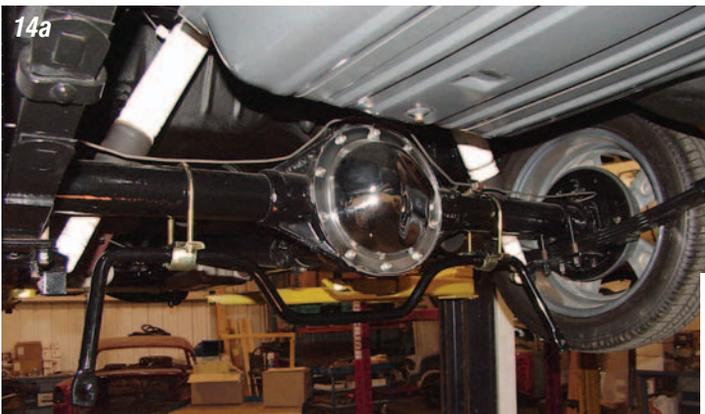
**Photos 14a & 14b:** Install the U-bolts, brackets, nuts, bushings and anti-sway bar onto the rear end housing allowing everything to hang loose at this time.
