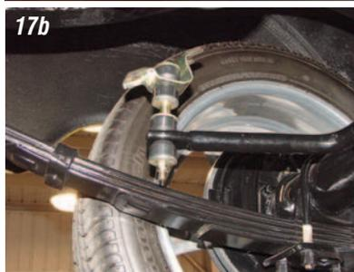
**Photos 17a, 17b & 17c:** Install the link kits and brackets onto the sway bar. With the car in the ride height position, place the mounting brackets on the bottom of the frame and mark the frame where the holes will need to be drilled.
