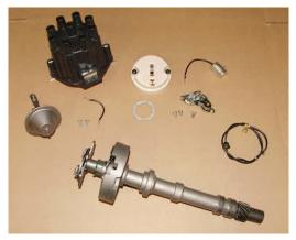
Photo 1: The distributor must be removed to install the HEI conversion kit. First remove the distributor cap, ignition rotor, points, condenser and points lead.
