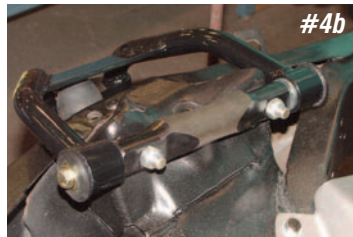
Photos #4a & #4b: The tubular upper control arms are where the geometry change takes place, substantially improving steering and handling. Two degrees more camber and five degrees more caster are built into the arms. This will allow the alignment shop to achieve any alignment specs that could possibly be required. The upper arms include ball joints, the cross shafts and urethane bushings.
