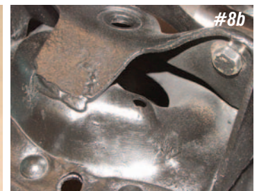
Photos #8a & #8b: The top end of the coil spring will seat into the upper coil spring pocket in the frame.
