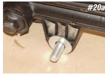
Photos #20a & #20b: On the driver's side of the rack and pinion unit there is a cast ear. A flat washer is used on the front and rear of the ear.
