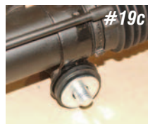
Photos #19a, #19b & #19c: The rack and pinion unit mounts to the crossmember with two 1/2" bolts. On the passenger side of the rack and pinion unit there is a sleeve with two bushings. A cupped washer is placed on the front side of the bushing and a flat washer on the back side.
