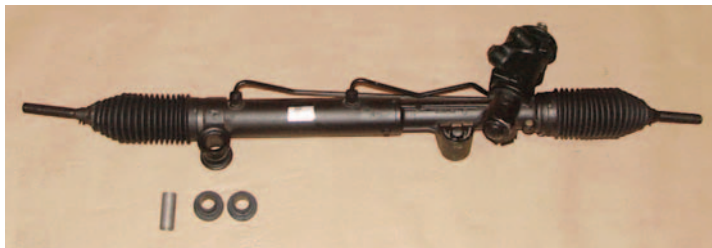
Photo #18: The rack and pinion unit is a power steering unit that originally fit a 1982 to 1990 Celebrity. This rebuilt and guaranteed unit is remanufactured just for CCI to accept the original 1955-57 outer tie rod ends and sleeves.
