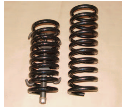
Photo #7: When installing front coil springs ALWAYS use a coil spring compressor. Using the spring compressor, collapse the coil spring about 2-1/2".
