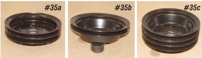
Photos #35a, #35b & #35c: A third track crankshaft pulley is supplied with the kit. This pulley will drive the power steering pump. The first groove on the crankshaft is for the generator or alternator, the second groove is for air conditioning. The third track pulley keys onto the front of a double groove crankshaft pulley P/N 51-03 (not supplied with kit).
