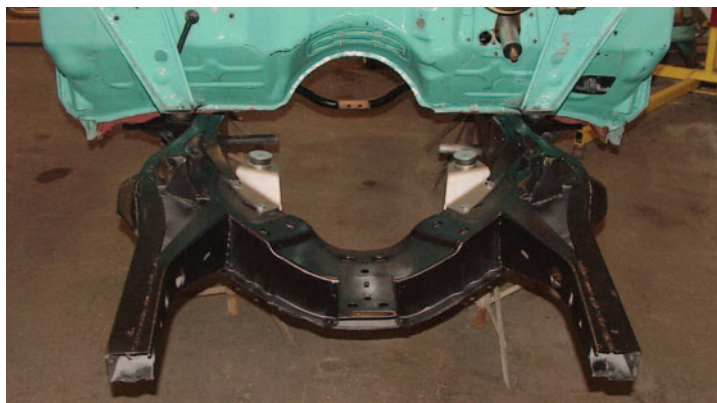
Photo #1: Here is truly a blank slate; a sand blasted and painted 1957 frame awaiting front suspension parts. A few hours with some hand tools and we will have a car that will handle like a dream.
