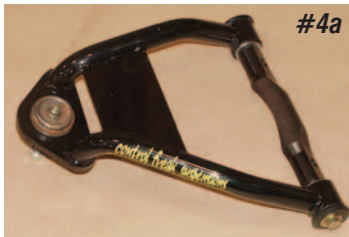
Photos #4a & #4b: The tubular upper control arms are where the geometry change takes place, substantially improving steering and handling. Two degrees more camber and five degrees more caster are built into the arms. This will allow the alignment shop to achieve any alignment specs that could possibly be required. The upper arms include ball joints, the cross shafts and urethane bushings.
