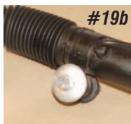
Photos #19a, #19b & #19c: The rack and pinion unit mounts to the crossmember with two 1/2" bolts. On the passenger side of the rack and pinion unit there is a sleeve with two bushings. A cupped washer is placed on the front side of the bushing and a flat washer on the back side.
