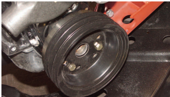
Photo #36: The crankshaft pulleys are held to the harmonic balancer with three 3/8" x 1" bolts for small block or big block.
