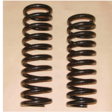
Photo #7: When installing front coil springs ALWAYS use a coil spring compressor. Using the spring compressor, collapse the coil spring about 2-1/2".
