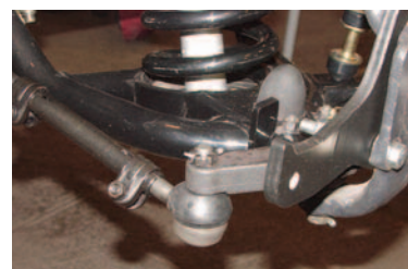
Photo #24: With the steering arms in place the outer tie rod ends can be installed. Tighten the tie rod end nuts and install the cotter pins.
