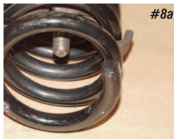
Photos #8a & #8b: The top end of the coil spring will seat into the upper coil spring pocket in the frame.
