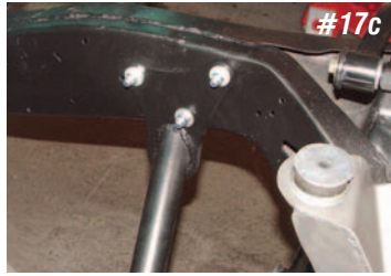
Photos #17a, #17b, #17c & #17d: The IFS kit includes the rack and pinion steering system. The rack and pinion unit is held in place with a tubular crossmember that bolts to the frame using the two holes
