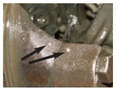
Photo 4: Before removing the two main caps, use a punch and hammer and mark the caps and case. Just like on an engine, the main caps must go back on the same way they came off.
