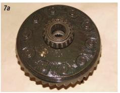
**Photos 7a, 7b & 7c:** The ring gear is held to the carrier with ten 5/8" X 1" right hand bolts. Using an air impact or pull bar, remove the bolts. Next, using a brass punch and hammer, carefully remove the ring gear from the carrier.
