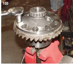
55 ft/lbs. A slick way to hold the carrier while torquing the ring gear bolts is to mount an axle in a vise and install the carrier onto the axle splines.
