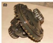
**Photos 6a & 6b:** With the main caps removed, the carrier and ring gear can be removed from the center section.
