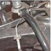
**Photo #10a & 10b:** A 3/16" X 50" brake line is supplied to connect the 3/16" tee to the right front wheel. The line can be routed across the front engine crossmember along with the other 3/16" line from the master cylinder.
