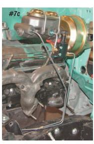
fitting screws into the front port of the master cylinder for the front brakes. The line is routed down to just behind the left upper control arm.
