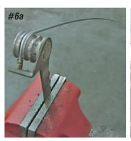
Photo #6a & 6b & 6c: The brake lines are supplied straight to allow the brake line kit to fit various applications. A 3/16" X 60" line with a 3/16" inverted flare union is supplied to connect the outlet port on the proportioning valve to the factory brake line on the passenger side of the car. Using a tubing bender like P/N
