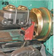
used with power brakes or manual brakes. The proportioning valve bracket is held in place with the two master cylinder mounting studs.
