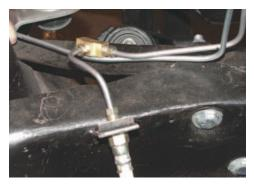
**Photo #9:** A 3/16" X 5" brake line is supplied to connect the 3/16" tee to the left front wheel.
