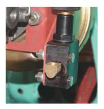
**Photo #4:** The proportioning valve is held to the valve bracket with two 1/4" X 1-1/4" bolts, nuts and lock washers **P/N 34-400.** Mount the valve with the adjusting knob facing upward and the inlet facing to the front of the master cylinder.
