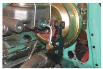
**Photo #5:** The brake line set **P/N 20-138** includes a short 90-degree 1/4" brake line that connects the rear port of the master cylinder to the inlet side of the proportioning valve.
