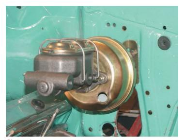
**Photo #1:** A dual master cylinder has two outlet ports. If an adjustable proportioning valve is going to be used, the front port of the master cylinder will be used for the front brakes and the rear port will be used for the rear brakes.
