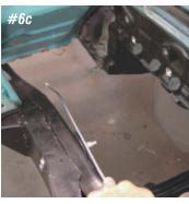
**49-38**, bend the brake line so that it is routed across the front engine crossmember and connects to the factory rear brake line near the base of the firewall on the passenger side.
