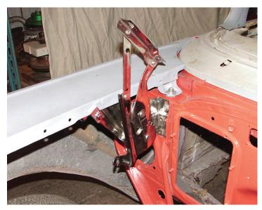
Photo 3: If you want to go that extra step, install the new polished stainless steel hood hinges P/N 54-31. With the new billet brackets and the stainless steel hinges, your '57 will look super custom under the hood! Good luck.
