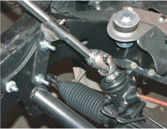
Photo #3: The new third U-joint support bracket bolts to the two forward bolts on the driver's side and supports the steering shaft.
