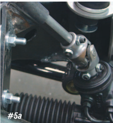
Photo #4: With the shaft installed in the column coupler and the new U-joint bracket, it must line up perfectly with the lower U-joint or the shaft will be in a bind.
