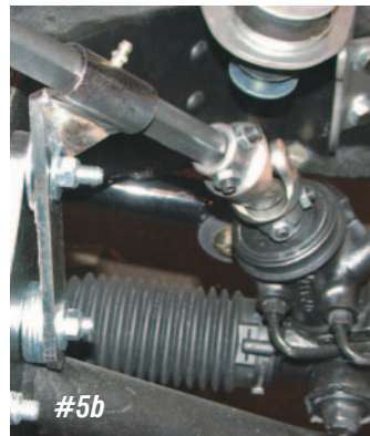
Photo #4: With the shaft installed in the column coupler and the new U-joint bracket, it must line up perfectly with the lower U-joint or the shaft will be in a bind.
