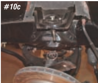
Photo #10a & 10b & 10c: With the load taken off the upper control arm, remove the cotter pin and nut from the upper ball joint. Using a ball joint pickle fork tool, disconnect the ball joint from the spindle.
