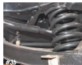
Photo #3a & 3b: If the upper control arms only are going to be changed, the brakes, steering and anti-sway bar can stay intact. Our customer wants lowering coil springs P/N 21-133 installed so all of these parts will need to be removed from the spindle. The anti-sway bar is connected the lower control arm with a 5/16" bolt, nut, bushings and washers.
