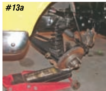
Photo #13a & 13b & 13c & 13d: To remove the coil springs, turn the tall nut on the spring compressor counterclockwise. This will allow the lower control arm to swing down. Place a floor jack under the lower ball joint nut to support the lower control arm as the nut on the spring compressor is turned. Lower the floor jack and remove the coil spring.
