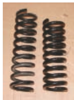
Photo #14: The 2" lowering coil springs P/N 21-133 are black powder coated and are 2-1/2" shorter than the stock coil springs, which will lower the car 2". The lowering springs have a 60 lb higher load rating than the stock coil spring for a better ride than just cutting a stock set of coil springs. These springs can be used with a small block or big block.
