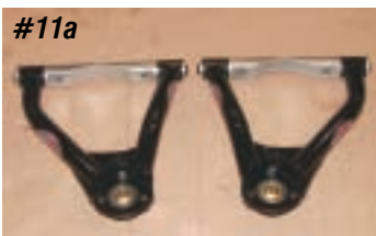
Photo #12a & 12b: The new upper control arms P/N 21-185 are black powder coated and have aluminum cross shafts and new ball joints. The new control arms have two degrees more positive camber and five degrees more positive caster. With the additional caster and camber, there will be no problem achieving the proper alignment specifications for any steering type. With the control arm in place, torque the control arm shaft nuts to 55 ft/lbs.
