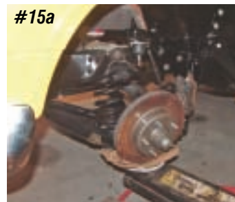
Photo #15a & 15b & 15c: Using only the floor jack to hold the lower control arm and coil spring in place, feed the coil spring compressor back up through the control arm and frame.
