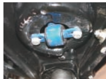
Photo #1a & 1b: First, remove the front shock absorber. The stud on the shock absorber is attached to the upper control arm stand with a 9/16" nut, cupped washer and rubber grommet.
