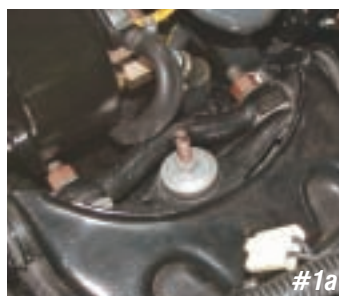
Photo #1a & 1b: First, remove the front shock absorber. The stud on the shock absorber is attached to the upper control arm stand with a 9/16" nut, cupped washer and rubber grommet.
