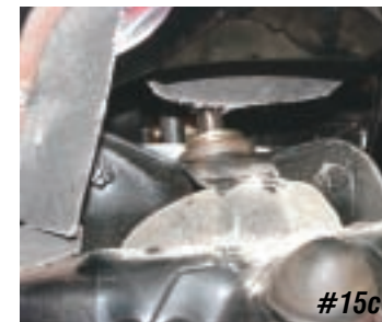
Photo #15a & 15b & 15c: Using only the floor jack to hold the lower control arm and coil spring in place, feed the coil spring compressor back up through the control arm and frame.
