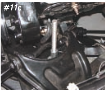
Photo #11a & 11b & 11c & 11d: The upper control arm is held to the upper control arm stand with two 7/16" nuts and lock washers. To remove the control arm on the drivers side, the power steering pump needed to be removed and moved inward away from the control arm. The header also needed to be removed. If the car had exhaust manifolds, they would not have needed to be removed. With the pump and header out of the way, remove the two 7/16" nuts and lock washers. Slide the control arm inward and lift it out through the engine compartment.
