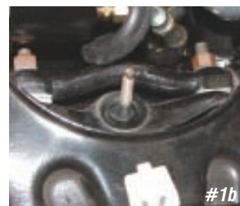
Photo #1a & 1b: First, remove the front shock absorber. The stud on the shock absorber is attached to the upper control arm stand with a 9/16" nut, cupped washer and rubber grommet.
