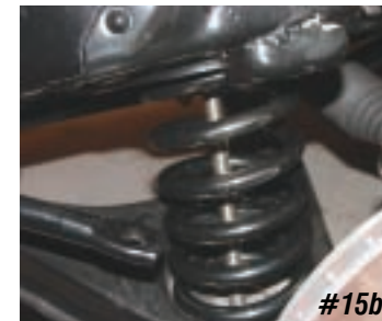
Photo #14: The 2" lowering coil springs P/N 21-133 are black powder coated and are 2-1/2" shorter than the stock coil springs, which will lower the car 2". The lowering springs have a 60 lb higher load rating than the stock coil spring for a better ride than just cutting a stock set of coil springs. These springs can be used with a small block or big block.
