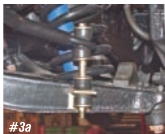
Photo #3a & 3b: If the upper control arms only are going to be changed, the brakes, steering and anti-sway bar can stay intact. Our customer wants lowering coil springs P/N 21-133 installed so all of these parts will need to be removed from the spindle. The anti-sway bar is connected the lower control arm with a 5/16" bolt, nut, bushings and washers.
