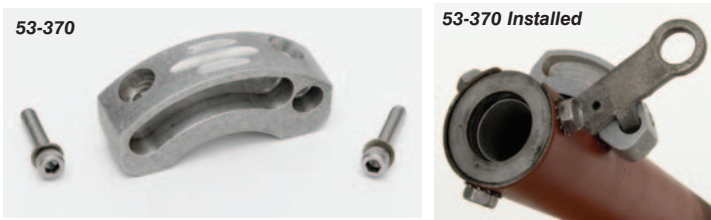
Photo #3a & 3b: There is more than enough room in the notch on the stock steering column mast jacket to allow the shift arm to travel far enough to operate a three or four-speed automatic transmission. If the original detent is modified to achieve the amount of travel needed to shift from overdrive to first gear, the original lower end of the detent will likely break off.
