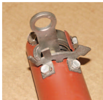
Photo #1: The original automatic steering column utilizes a bolt-on shifter detent at the bottom of the column available as P/N 19-38 or 19-39. This detent positively locks the column shift arm in the "Park" position, keeping the transmission safely locked into "Park".
