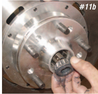
Photo #11a & 11b: Next install the rotor onto the spindle. Make sure the inner bearing and seal slides all the way onto the spindle and install the outer bearing.
