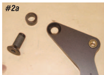
Photo #2a & 2b & 2c: A 5/8 X 1" countersunk bolt is used at the top to hold the bracket in place. A 1/2" spacer is installed between the top of the bracket and spindle. Leave this bolt loose at this time.
