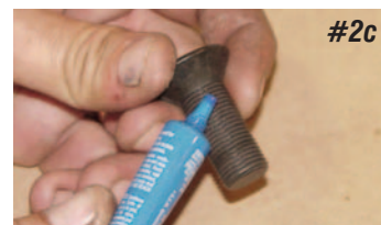
Photo #2a & 2b & 2c: A 5/8 X 1" countersunk bolt is used at the top to hold the bracket in place. A 1/2" spacer is installed between the top of the bracket and spindle. Leave this bolt loose at this time.
