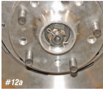
Photo #12a & 12b: The stock drum brake spindle nuts are used with the Wilwood disc brake kit. Install a new spindle washer (supplied with the kit) and torque the spindle nut to 30 to 33 ft/lbs and turn counterclockwise until the cotter pin lines up with the hole in the spindle and install a new cotter pin. Place a small amount of grease on the O-ring and threads of the screw-on dust cap and screw the cap on until it bottoms out.
