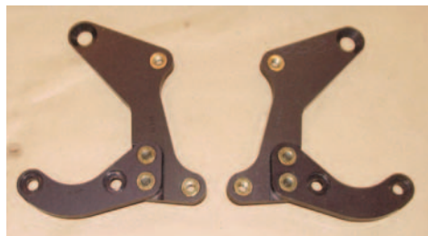
Photo #1: The disc brake brackets are a two-piece bracket that will be assembled and bolted to the stock '55-'58 spindles using the factory
