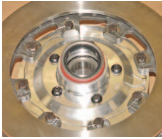
Photo #10: Install the inner bearing and seal. The seal is driven in flush with the back of the hub.
