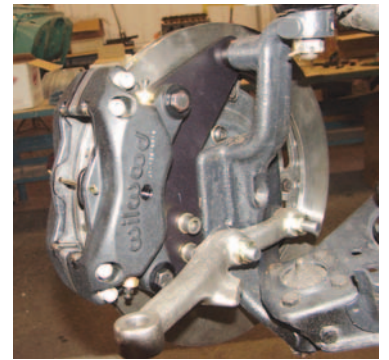
Photo #14: The caliper has two mounting ears that match up to the two threaded holes in the main mounting bracket. The caliper is bolted to the main bracket with two 3/8" X 1" bolts and lock washers. The caliper may require lateral shimming to achieve the proper clearance between the brake pads and the rotor. Mount the caliper to the main bracket using the two bolts and lock washers. Do not use any thread locker at this time.
