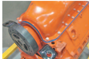
Photo #7a & 7b: The one-piece oil pan gasket will just about fall into place. All of the oil pan bolt holes and the dipstick hole will line up perfectly. Installation is a breeze even if the engine is in the car. When installing the silicone oil pan gasket, no gasket sealer is needed.
