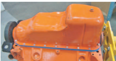
Photo #7a & 7b: The one-piece oil pan gasket will just about fall into place. All of the oil pan bolt holes and the dipstick hole will line up perfectly. Installation is a breeze even if the engine is in the car. When installing the silicone oil pan gasket, no gasket sealer is needed.
