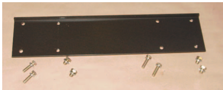
Photo #2a & 2b: The front of the seat tracks have a "foot" that fits under clips P/N 35-51 that is bolted to the forward floor seat brace. At the rear of the seat, the track has two holes that bolt directly to the floor.
