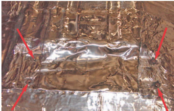
Photo #1: The factory bench seat is bolted to the floor of the car with four 5/16" bolts per side. There are four nut inserts per side welded to the seat brace under the floor that the bolts thread into.
