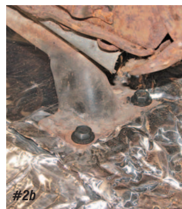
Photo #2a & 2b: The front of the seat tracks have a "foot" that fits under clips P/N 35-51 that is bolted to the forward floor seat brace. At the rear of the seat, the track has two holes that bolt directly to the floor.
