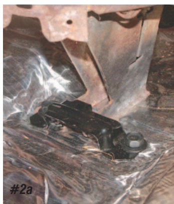
Photo #2a & 2b: The front of the seat tracks have a "foot" that fits under clips P/N 35-51 that is bolted to the forward floor seat brace. At the rear of the seat, the track has two holes that bolt directly to the floor.
