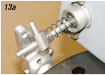
Photo #13a & 13b: The master cylinder is equipped with a threaded pushrod. The 3" long spring provided should be installed onto the pushrod shaft first. Screw the coupler onto the shaft to connect the master cylinder pushrod to the clutch pedal arm. Make sure the flat side on the coupler is facing away from the master cylinder.
