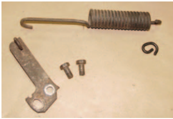
Photo #4: The stock clutch pedal swing arm has a return spring and bracket that will need to be removed. The return spring bracket is bolted to the clutch pedal arm with two 9/16" bolts.
