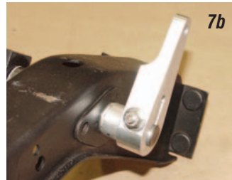
Photo #7a & 7b: Install the aluminum bushing in the kit onto the clutch arm shaft. Next install the billet aluminum clutch master cylinder arm. Make sure the offset of the arm is toward the left (driver side) of the pedal assembly. The arm is held to the shaft with an Allen head bolt and lock nut that will pass over the flat cut in the clutch pedal shaft just like the original arm.
