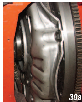
Photo #30a & 30b: Once all the air has been removed, the release bearing will move forward 1/2" to disengage the clutch. This amount of movement is enough to adequately disengage a three finger or diaphragm style pressure plate.
