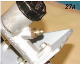
Photo #27a & 27b: The 90-degree end on the hose from the release bearing connects to the #4 fitting on the master cylinder.
