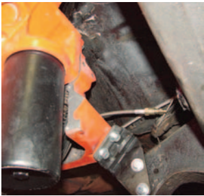
Photo #26: The supply hose can be routed through the firewall in any desired location. Make sure the hose is kept away from any moving parts or hot exhaust. The kit includes a grommet so that the hose will be protected as it passes through the firewall.
