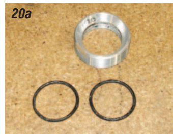
Photo #20a & 20b: The adjusting collar for the release bearing has two o-rings on the inside bore so that it will not spin. Lubricate the o-rings with a light oil and install the collar onto the front bearing retainer. The beveled side of the collar installs against the transmission face.
