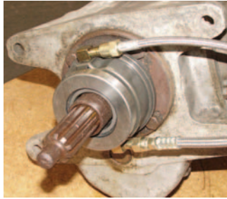
Photo #28a, 28b & 28c: With everything installed it is time to put brake fluid in the clutch master cylinder. Use ONLY DOT 3 brake fluid and not silicone brake fluid. Using silicone brake fluid will damage the release bearing and void any warranty. If the gauge cluster is removed, there is room to get a container of brake fluid up to the master cylinder top to fill the master cylinder. Fill it to within 1/2" of the top. If there is not enough room to get a container of brake up to the master cylinder use the supplied squeeze ball and hose to fill the master cylinder. Spread a garbage bag out on the floor of the car to protect the carpet.
