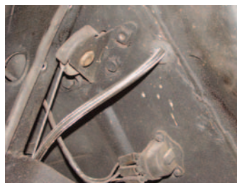
Photo #26: The supply hose can be routed through the firewall in any desired location. Make sure the hose is kept away from any moving parts or hot exhaust. The kit includes a grommet so that the hose will be protected as it passes through the firewall.
