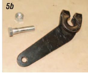
Photo #5a & 5b: The clutch pedal pushrod arm is splined to the clutch pedal shaft and secured with a 9/16" bolt, nut and lock washer. The stock arm will be replaced with a new billet arm for the hydraulic master cylinder.
