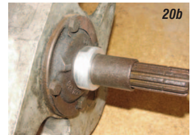
Photo #20a & 20b: The adjusting collar for the release bearing has two o-rings on the inside bore so that it will not spin. Lubricate the o-rings with a light oil and install the collar onto the front bearing retainer. The beveled side of the collar installs against the transmission face.
