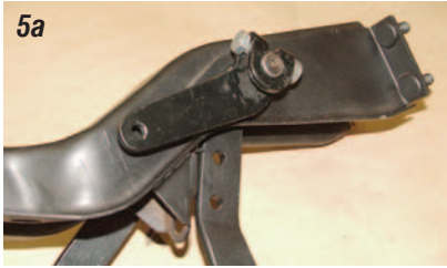
Photo #5a & 5b: The clutch pedal pushrod arm is splined to the clutch pedal shaft and secured with a 9/16" bolt, nut and lock washer. The stock arm will be replaced with a new billet arm for the hydraulic master cylinder.
