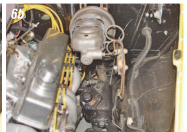
Photos 6a & 6b: The steering box is removed through the top of the engine compartment. Our project car has the alternator mounted on the front two header bolts on the driver's side and a power brake booster and dual master cylinder – all in the way! We will remove the alternator to make removing the steering box easier. With the alternator out of the way, there is plenty of room to remove the steering box.
