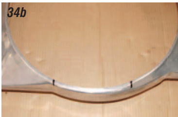
Photos 34a & 34b: A third track pulley must be added to the crankshaft to drive the power steering pump. By adding a third track pulley to the crankshaft, the fan shroud will need to be notched. Mark the shroud and remove.
