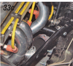
Photos 33a, 33b & 33c: The upper bearing in the steering column P/N 53-21 was bad so this was the perfect time to change it before we installed the steering shaft, the steering wheel adapter and the intermediate with U-joints. With everything set and the screws on the U-joints locked down, we had a 1/16" gap between the steering wheel adapter and the top of the steering column. This gap will keep the steering wheel adapter from touching the painted surface of the turn signal housing.
