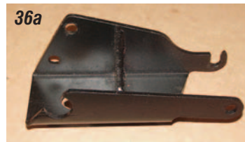
Photos 36a & 36b: The power steering pump mounts to the front of the engine down low on the driver's side. The pump mounting bracket P/N 53-27 or 53-27C can be used as the power steering pump mounting bracket on cars with side engine mounts or as a combination front engine mounting bracket and pump mounting bracket on engines with front mounts.
