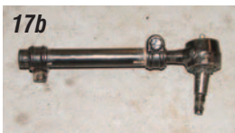
Photos 17a, 17b & 17c: The Eckler's Classic Chevy Rack and Pinion Kit utilizes the original outer tie rod ends and adjusting sleeves so there are no metric parts installed on your Classic! The outer tie rod ends and adjusting sleeves were in perfect shape on our project car so we will reuse them. If they were bad, the adjusting sleeves are available new as P/N 21-08 and the outer tie rod ends P/N 21-07 . Install the adjusting sleeves and tie rod ends and set the toe in as close as you can for now. Once the rack and pinion is completely installed, the car will need to be taken to the alignment shop.
