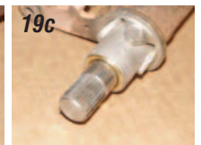
Photos 19a, 19b & 19c: The rack & pinion kit includes two large brass bushings. One of the two bushings will fit into the bottom of the original mast jacket to support the lower end of the new steering shaft. Choose the correct size bushing that will slide up into the bottom of the mast jacket and drive the bushing in so that it is flush with the bottom of the tube.
