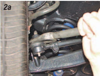
Photos 2a & 2b: First, we will disconnect the outer tie rod ends from the steering knuckles (outer steering arms). Remove the cotter pin and nut from the tie rod end and using a tie rod splitter and disconnect the tie rod ends from the steering arms. If the outer tie rod ends and adjusting sleeve are in good shape, they will be reused with the rack and pinion.
