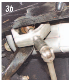
Photos 3a, 3b & 3c: The pitman arm is held to the steering box with a 1-5/16" right hand thread nut and lock washer. Using a socket and breaker bar or impact wrench, remove the nut and lock washer. Next using a pitman arm puller and a breaker bar or impact, remove the pitman arm from the steering box.
