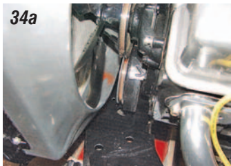
Photos 34a & 34b: A third track pulley must be added to the crankshaft to drive the power steering pump. By adding a third track pulley to the crankshaft, the fan shroud will need to be notched. Mark the shroud and remove.
