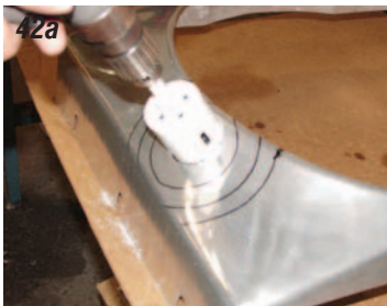
Photos 42a & 42b: First, drill a 1-3/4" hole at the center of the markings to line up with the power steering pump shaft when the pump is adjusted as far out as it will go.
