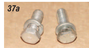
Photos 37a & 37b: The pump bracket P/N 53-27 (small block short water pump) is held to the front of the engine with two 3/8" X 3/4" bolt and lock washers provided.
