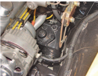
Photo 1: The original steering box mounts to the frame just behind the upper control arm with three carriage bolts. When installing the rack, all the steering linkage should be removed.
