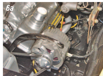
Photos 6a & 6b: The steering box is removed through the top of the engine compartment. Our project car has the alternator mounted on the front two header bolts on the driver's side and a power brake booster and dual master cylinder – all in the way! We will remove the alternator to make removing the steering box easier. With the alternator out of the way, there is plenty of room to remove the steering box.
