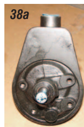
Photos 38a, 38b & 38c: The power steering pump P/N 53-28 is held to the bracket with a 3/8" X 3/4" bolt and lock washer in front and a stud at the rear that uses a 3/8" flat washer, lock washer and nut provided with the bracket. With the pump in place, we now see that the shroud will need to be trimmed for the power steering pump pulley. This would be true with a big block or small block engine.
