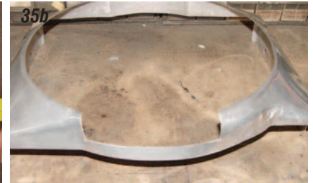
Photos 35a & 35b: Future plans include adding air conditioning, so we will install a double groove pulley along with the third track pulley on the balancer. All three pulleys together measure 1-3/4" deep. Using the marks on the fan shroud as the reference point, cut a 1-3/4" deep notch in the shroud. A fine tooth hack saw or tin snips works great to cut the aluminum shroud.
