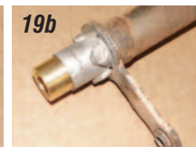
Photos 19a, 19b & 19c: The rack & pinion kit includes two large brass bushings. One of the two bushings will fit into the bottom of the original mast jacket to support the lower end of the new steering shaft. Choose the correct size bushing that will slide up into the bottom of the mast jacket and drive the bushing in so that it is flush with the bottom of the tube.
