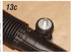
Photos 12a, 12b & 12c: The rack and pinion unit is bolted to the crossmember with two 1/2" X 3" bolts and washers. The driver's side of the rack and pinion has a cast ear where a 1/2" flat washer is installed on each side of the ear.
