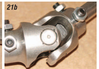
Photos 21a & 21b: The U-joints are held to the intermediate shaft with set screws and jam nuts. Make sure when the shaft is installed in the U-joint that the shaft does not protrude past the inside of the yoke. If it does, the shaft will make contact with the opposing yoke of the U-joint and create a bind.
