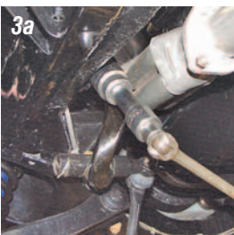
Photos 3a, 3b & 3c: The pitman arm is held to the steering box with a 1-5/16" right hand thread nut and lock washer. Using a socket and breaker bar or impact wrench, remove the nut and lock washer. Next using a pitman arm puller and a breaker bar or impact, remove the pitman arm from the steering box.
