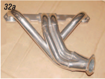
Photos 32a & 32b: We have removed the left hand header only and replaced it with the Eckler's Classic Chevy 3/4-length header P/N 24-53C-LH. This header can be purchased as a pair P/N 24-53 (uncoated) or P/N 24-53C (coated). The #24-53 headers will work with stock front mounts or any brand side mounts, automatic column shift or manual transmissions, with or without mechanical clutch linkage and with either straight or angle plug heads. With the #24-53 headers there is plenty of room for the lower U-joint and shaft on the driver's side.
