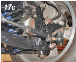
Photos 17a, 17b & 17c: The Eckler's Classic Chevy Rack and Pinion Kit utilizes the original outer tie rod ends and adjusting sleeves so there are no metric parts installed on your Classic! The outer tie rod ends and adjusting sleeves were in perfect shape on our project car so we will reuse them. If they were bad, the adjusting sleeves are available new as P/N 21-08 and the outer tie rod ends P/N 21-07 . Install the adjusting sleeves and tie rod ends and set the toe in as close as you can for now. Once the rack and pinion is completely installed, the car will need to be taken to the alignment shop.
