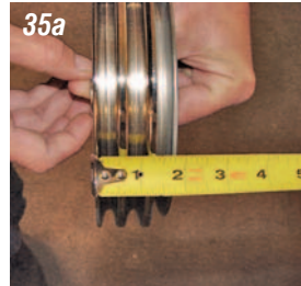
Photos 35a & 35b: Future plans include adding air conditioning, so we will install a double groove pulley along with the third track pulley on the balancer. All three pulleys together measure 1-3/4" deep. Using the marks on the fan shroud as the reference point, cut a 1-3/4" deep notch in the shroud. A fine tooth hack saw or tin snips works great to cut the aluminum shroud.
