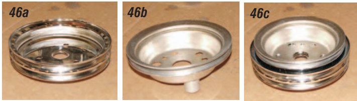
Photos 46a, 46b, 46c & 46d: The first groove on our balancer pulleys closest to the harmonic balancer will drive the water pump and alternator. The second groove is for the water pump and air conditioning compressor and the third groove runs the power
