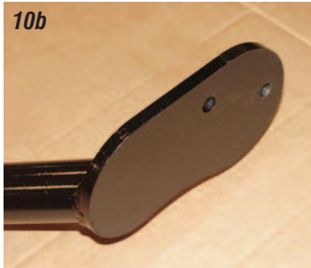
Photos 10a & 10b: The rack and pinion crossmember bolts to the frame on the driver's side using the stock holes for the steering box. On the passenger side, the crossmember bolts to the frame using the original holes for the idler arm.
