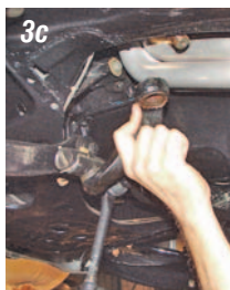
Photos 3a, 3b & 3c: The pitman arm is held to the steering box with a 1-5/16" right hand thread nut and lock washer. Using a socket and breaker bar or impact wrench, remove the nut and lock washer. Next using a pitman arm puller and a breaker bar or impact, remove the pitman arm from the steering box.
