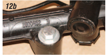
Photos 12a, 12b & 12c: The rack and pinion unit is bolted to the crossmember with two 1/2" X 3" bolts and washers. The driver's side of the rack and pinion has a cast ear where a 1/2" flat washer is installed on each side of the ear.
