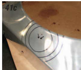
Photos 41a, 41b & 41c: When the power steering pump was installed, the shaft made a mark on the shroud. Using the two marks that were made with the pulley template, center the template on the scratch that the pump shaft made and mark the outer circumference of the template. Next, make several small diameter marks on the shroud to be used as reference points when trimming the shroud.
