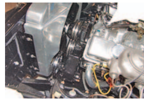
Photo 50: Now you may install the fan shroud for the last time. The legs on the shroud get trapped between the core support and the radiator to finish things off.
