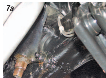
Photos 7a & 7b: Remove the three nuts, lock washers and carriage bolts and the steering box can be removed from the car.
