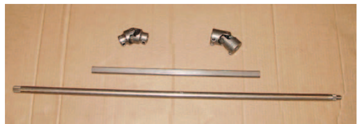
Photo 20: When using an original steering column, a new shaft steering shaft kit is supplied with the rack and pinion kit. This includes the column shaft, the intermediate shaft and upper and lower U-joints.
