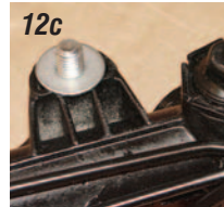
Photos 12a, 12b & 12c: The rack and pinion unit is bolted to the crossmember with two 1/2" X 3" bolts and washers. The driver's side of the rack and pinion has a cast ear where a 1/2" flat washer is installed on each side of the ear.
