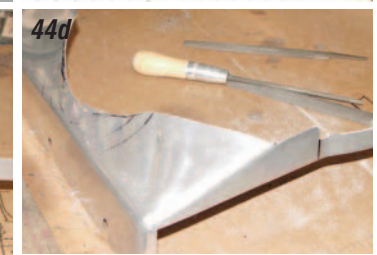
Photos 44a, 44b, 44c & 44d: With the pump and the single groove power steering pump crankshaft pulley P/N 53-34 installed, you can see that the fan shroud is in the way of the belt. Mark the shroud where the fan belt is going to travel and once again remove the shroud and trim it for the power steering pump belt.
