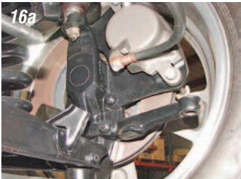
Photos 16a & 16b: The original steering arms are bolted to the spindles with two 7/16" bolts and nuts. Remove the two nuts and install the new arms.
