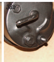
Photos 38a, 38b & 38c: The power steering pump P/N 53-28 is held to the bracket with a 3/8" X 3/4" bolt and lock washer in front and a stud at the rear that uses a 3/8" flat washer, lock washer and nut provided with the bracket. With the pump in place, we now see that the shroud will need to be trimmed for the power steering pump pulley. This would be true with a big block or small block engine.
