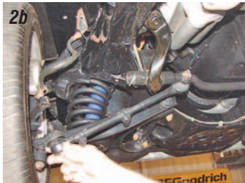
Photos 2a & 2b: First, we will disconnect the outer tie rod ends from the steering knuckles (outer steering arms). Remove the cotter pin and nut from the tie rod end and using a tie rod splitter and disconnect the tie rod ends from the steering arms. If the outer tie rod ends and adjusting sleeve are in good shape, they will be reused with the rack and pinion.
