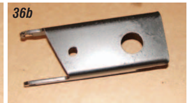
Photos 36a & 36b: The power steering pump mounts to the front of the engine down low on the driver's side. The pump mounting bracket P/N 53-27 or 53-27C can be used as the power steering pump mounting bracket on cars with side engine mounts or as a combination front engine mounting bracket and pump mounting bracket on engines with front mounts.
