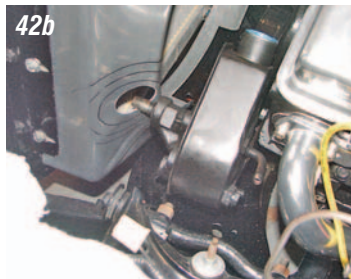
Photos 42a & 42b: First, drill a 1-3/4" hole at the center of the markings to line up with the power steering pump shaft when the pump is adjusted as far out as it will go.
