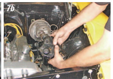
Photos 7a & 7b: Remove the three nuts, lock washers and carriage bolts and the steering box can be removed from the car.
