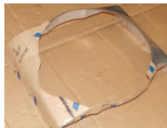
Photo 45: Before we installed the fan shroud for the last time, we made a template of the cut-outs on the shroud. If you go to our website www.classicchevy.com and pull up either P/N 18-306 or P/N 18-307 fan shroud, you can download the template. Or if you wish you can send a self-addressed envelope attn: CCI Tech Dept Fan Shroud Template and we will be glad to send you a copy.
