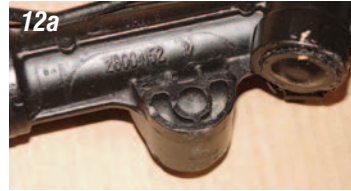
Photos 12a, 12b & 12c: The rack and pinion unit is bolted to the crossmember with two 1/2" X 3" bolts and washers. The driver's side of the rack and pinion has a cast ear where a 1/2" flat washer is installed on each side of the ear.
