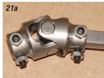
Photos 21a & 21b: The U-joints are held to the intermediate shaft with set screws and jam nuts. Make sure when the shaft is installed in the U-joint that the shaft does not protrude past the inside of the yoke. If it does, the shaft will make contact with the opposing yoke of the U-joint and create a bind.
