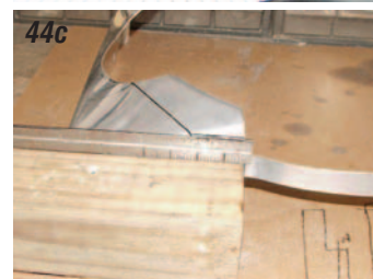
Photos 44a, 44b, 44c & 44d: With the pump and the single groove power steering pump crankshaft pulley P/N 53-34 installed, you can see that the fan shroud is in the way of the belt. Mark the shroud where the fan belt is going to travel and once again remove the shroud and trim it for the power steering pump belt.
