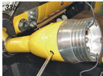
Photos 33a, 33b & 33c: The upper bearing in the steering column P/N 53-21 was bad so this was the perfect time to change it before we installed the steering shaft, the steering wheel adapter and the intermediate with U-joints. With everything set and the screws on the U-joints locked down, we had a 1/16" gap between the steering wheel adapter and the top of the steering column. This gap will keep the steering wheel adapter from touching the painted surface of the turn signal housing.
