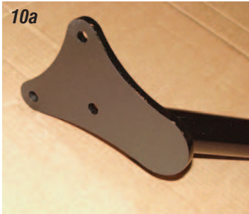
Photos 10a & 10b: The rack and pinion crossmember bolts to the frame on the driver's side using the stock holes for the steering box. On the passenger side, the crossmember bolts to the frame using the original holes for the idler arm.
