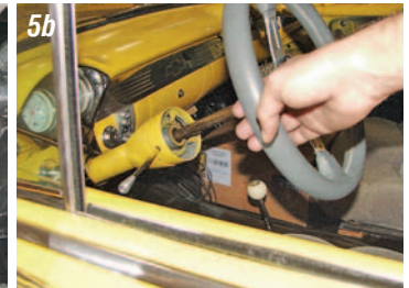
Photos 5a & 5b: The steering shaft that connects the steering wheel to the steering box is part of the steering box and not removable. To remove the steering box and shaft, the mast jacket (steering column) must be removed. If you are not planning on saving the old steering box, the shaft can be cut at the steering box to save you from removing the mast jacket from the car. This will save you some time and keep you from possibly scratching the paint in the dash area. With the steering shaft cut, the steering wheel and shaft will slide out the top of the mast jacket.
