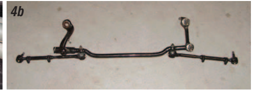
Photos 4a & 4b: The idler arm is located on the passenger side of the car and is held to the frame with two carriage bolts, nuts and lock washers. Remove the two nuts and lock washers and the entire steering linkage can be removed from the car.
