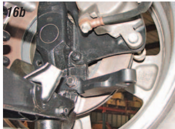
Photos 16a & 16b: The original steering arms are bolted to the spindles with two 7/16" bolts and nuts. Remove the two nuts and install the new arms.
