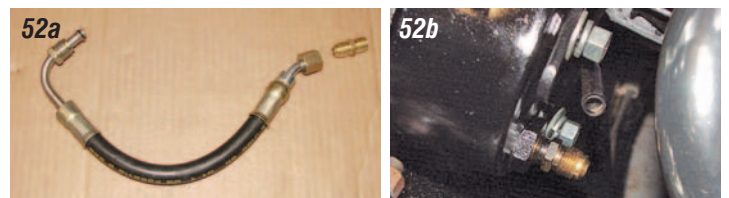
Photos 52a & 52b: The pressure hose P/N 53-38 (small block) or P/N 53-74 (big block) has a brass fitting on the end where it attaches to the pump and an 18 millimeter male O-ring fitting where it attaches to the rack and pinion. The brass fitting screws into the female inverted hole in the back of the pump.
