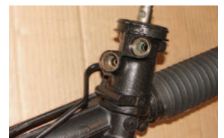
Photo 54: The 18 millimeter pressure port on the rack and pinion is to the left of the input shaft while the 16 millimeter return port is to the right of the input shaft.
