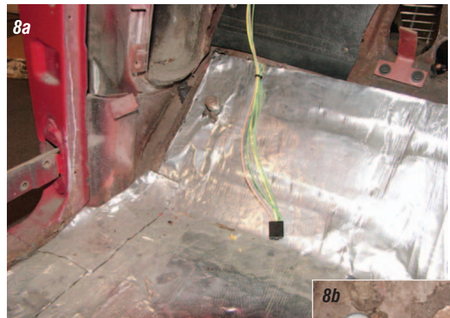
Photos 8a & 8b: The wires for the dimmer switch exit out the bottom of the fuse box and just about fall into place. The original dimmer switch on a 1955 and 1956 mounts from the outside toe board and is held in place with two 1/4" bolts. The new dimmer switch mounts to the inside of the toe board. The original 1/4" bolts can be used, but nuts will need to be used on the outside of the toe board to hold the switch in place.
