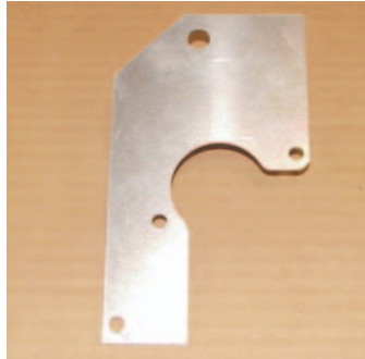
Photo 4: The fuse box is a bolt-in unit, unlike other kits. If your firewall is all painted, you don't want to go drilling holes. An aluminum bracket is attached to the firewall and the fuse box bolts right to it.
