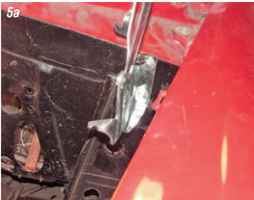
Photos 5a, 5b & 5c: The hood hinge is held to the firewall with two 3/8" bolts. The lower mounting bolt for the hinge will be replaced with a supplied 3/8" X 2 1/2" bolt. This longer bolt provides a mounting point for the fuse box bracket. There is a 5/16" hole about 4" below the lower hood hinge bolt, which is used for one of the firewall pad retainers. Remove the retainer and install the 1/4" X 2 1/2" straight screw. This screw will be used as the firewall retainer and as another mounting point for the fuse box bracket.
