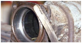
After the axle and backing plate were removed, the axle flange was cleaned off with a wire brush. It would also be good to clean the axle flange and bearing cup with a strong cleaner such as lacquer thinner or acetone.
