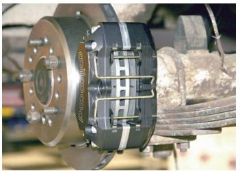
After the BP-10 Smart pads were loaded into the caliper, they were held in place with the quick-clip retainer. It is also important that the radius of the rotor matches the radius of the brake pads as seen here.
