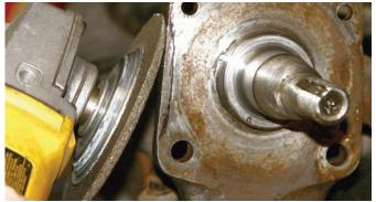
The spindle requires a small modification to get the caliper bracket to bolt on. Following the clearance line that was drawn on the spindle, a small radius was ground into the spindle base as seen here. This can be done with a small electric grinder and a hard disc.
