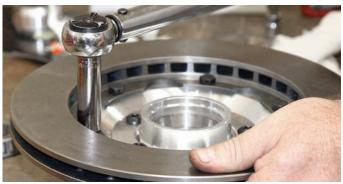
All of the rotor assembly bolts were coated with Loctite 271 and the hub to rotor bolts were tightened to 180 inlbs using an inch-pound torque wrench. The rotor-toadapter bolts were tightened to 35 ft-lbs using a foot-pound torque wrench.
