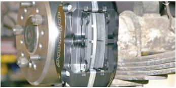
After the caliper is centered over the rotor, the BP-10 Smart Pads can be installed. Here they are being installed from the top of the Caliper. This design makes future pad changes very easy.
