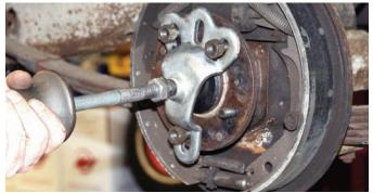
The axle wasn't going to come out without assistance so a slide hammer style puller was hooked up to release the bearing from the housing. The same procedure was also done on the other side of the differential.
