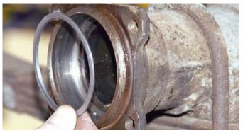
The '57 Chevy rear axle housing is a little different than the '55 and '56 Chevy housings. Because of that this spacer ring has to be used.
