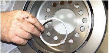
This installation requires another spacer ring that will allow this rotor to be seated on the Chevy axle.
