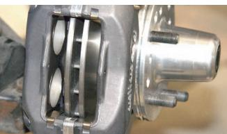
The caliper was attached to the caliper bracket to see if the rotor is centered. Installing or removing shims between the caliper and caliper bracket are used to make the adjustments necessary to get the rotor centered.
