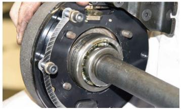
Here is the rear of the brake assembly with the bolts protruding through. The bolts will have to be lined up with the holes in the axle flange. Notice the caliper bracket is part of the parking brake assembly.
