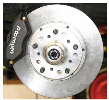
Here is the finished brake assembly with the Caliper mounted and ready to go. Before that is done the brake line was hooked up.
