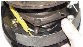
The brake system being installed has small inner parking brakes that have shoes similar to the original drum brakes. Here the holes in the bearing retainer are being lined up with the holes in the parking brake mechanism. The original square-head bolts were cleaned up and are being reused.
