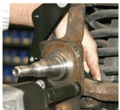
The two lower bracket bolts were connected with an impact gun and an open-end wrench.
