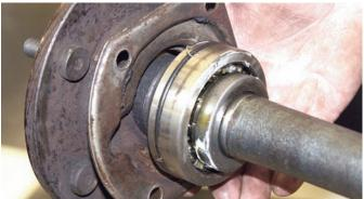
Another reminder, when the axles are out of the car it would be a good time to change the axle bearings if they have been in the car for a several years. If they have been changed recently you don't have to worry about it.
