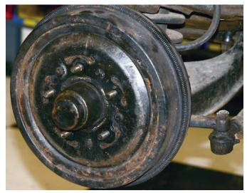
The Tri-year Chevys came with four-wheel drum brakes in manual form, or for a few dollars more you could get power brakes. If you have ever driven a '55 through '57 Chevy with original brakes they were marginal at best and when it was raining, the brakes would become magical, they would disappear.
