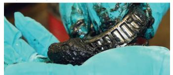
All of the bearings were packed with high temperature disc brake bearing grease. The large bearings were installed in the rear of the hub and then the grease seal was installed.
