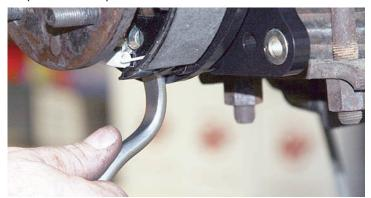
Using a brake spoon, the spanner ring should be turned until the little brake shoes are in close proximity to the rotor drum.
