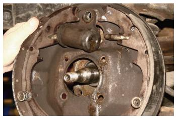
The backing plate may be stuck to the centering ring so it will have to be moved side to side to break it loose.
