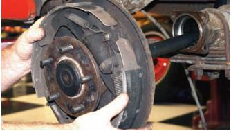
The axle and brake backing plate were removed from the assembly. This would be a good time to replace the axle bearings if they are original equipment or just worn out.
