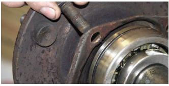
The special square-shaped axle bolts were removed and they should be cleaned up before they are reused. Save the nuts and washers because they will also be reused.
