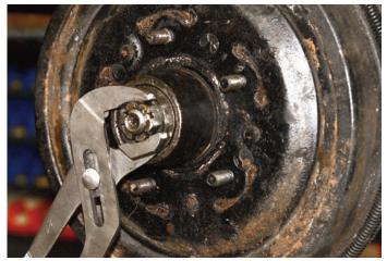
The cotter key was removed from the castle nut. Using the same large channel lock pliers the spindle nut was disconnected followed by the large flat washer.
