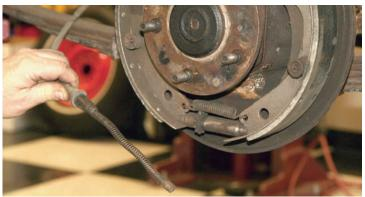
The backing plate and brake shoes will be removed as a unit but, before that can be done, the emergency brake cables were disconnected and removed from the assembly.
