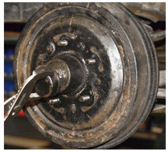
The dust was removed to access the front spindle nut. This cap was removed with large channel lock pliers.
