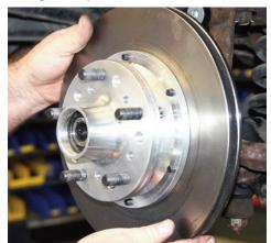
The rotor was placed onto the spindle making sure the small bearing was installed. The rotor was pushed back until the rotor was seated at the rear.
