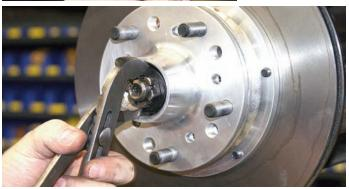
The large flat washer was installed and then the spindle nut was screwed into place. The nut was tightened until it was snug, but not overly tight. If the nut is too tight it will cause premature bearing failure.
