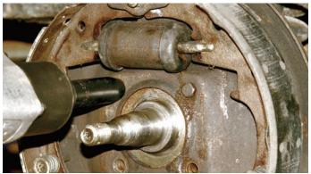
After the two lower bolts were disconnected and removed, the two upper bolts could be disconnected. Using an impact gun and an open-end wrench, the bolts were removed.
