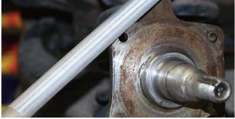
The grinding leaves rough edges so they were filed smooth before the bracket was bolted on.
