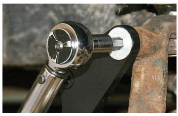
The upper Allen bolt was tightened to 77 ft-lbs using a footpound torgue wrench and an Allen head socket.
