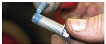
After the caliper was centered, the mounting bolts were coated with Loctite 271 and then they were reinstalled. Notice the bolt is used with a thick flat washer.
