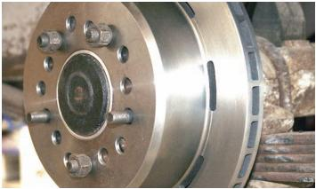
After the rotor was placed onto the axle flange centering ring it was secured with three lug nuts. There are three sets of holes in this rotor so make sure to use the proper set. A small mark by one of the holes will make it easy to figure out which one to use for your application.
