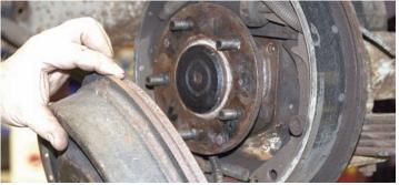
After the linings were backed off just a little, the brake drums were removed to access the brake assembly and backing plate.
