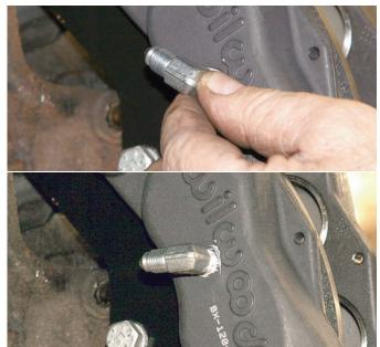
The caliper inlet fitting threads were coated with Teflon tape and then it was screwed into the caliper.
