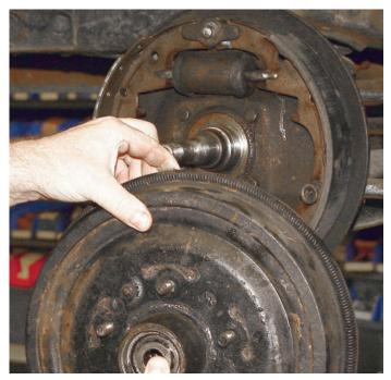
The drum was removed from the front spindle and was placed out of the way. If the drum is difficult to remove you may have to back off the brake shoes for more shoe to drum clearance.
