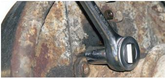
The four bolts that secure the backing plate to the axle flange were disconnected. The same bolts also secure the axle retainers, so at this point the axles can be removed.
