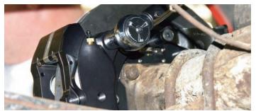
The caliper was placed over the rotor and the bolts were installed. Here one of the bolts is being tightened with a ratchet wrench. At this point the axle to rotor centering can be done before the bolts are secured. After the caliper is centered over the rotor the two mounting bolts can be tightened to 35 ft-lbs.
