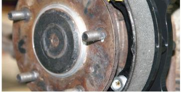
The spacer is loaded over the original centering ring as seen here. This small spacer needed to align the rotor. This is only used for alignment because the wheels and lug nuts will keep the rotor in place.
