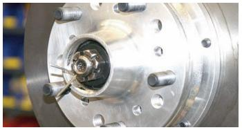
After the nut was snug, the castle portion of the nut was lined up with the hole in the spindle and then a cotter key was installed. The ends of the cotter key were bent to a point where they will not interfere with the dust cap installation.
