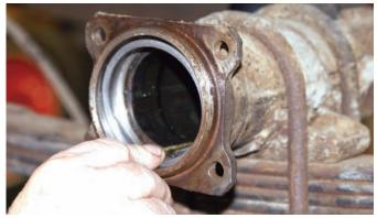
The spacer ring should be placed inside of the axlebearing cup. It was pushed back until is seated.
