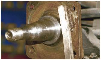
The spindle was cleaned off with a wire brush and then it was wiped down with lacquer thinner in preparation of installing the caliper bracket and rotor.
