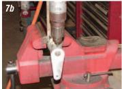
**Photos 7a & 7b:** The arm can be used as a guide to drill the required 3/16" hole. With the clutch arm in place, drill a 3/16" hole all the way though the clutch shaft.
