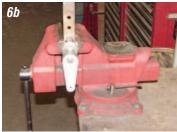
**Photos 6a & 6b:** Install the clutch pedal pivot sleeve and the spacer that is supplied with the hydraulic clutch system onto the clutch shaft. Next, install the arm onto the clutch shaft. The clutch shaft will protrude through the arm about 1/16". The arm installs so it is parallel with the clutch pedal arm.
