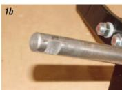
**Photos 1a & 1b:** The original clutch linkage arm for the mechanical clutch linkage was held to the clutch pedal shaft with a squeeze bolt. The bolt passes over a flat in the clutch pedal shaft and when tightened will squeeze the arm tight on the shaft.
