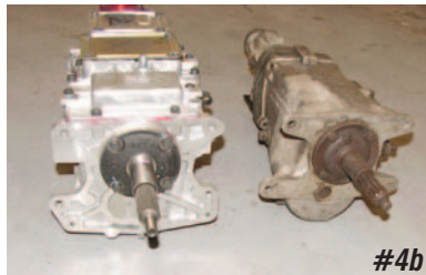
Photo #4a & 4b: The Tremec transmission is 1-3/4" longer than the Muncie transmission, so once the installation is complete, the driveshaft will need to be shortened accordingly. The Tremec has the same bellhousing bolt pattern as the Muncie so it is compatible with a stock Tri-Five bellhousing. The old cast iron manual transmission bellhousing is a bit archaic so we will use an all-new aluminum bellhousing.
