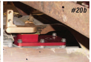
Photo #20a & 20b: The offset shifter base bolts to the top of the transmission using the six bolts that mounted the stock shifter base. Photo (a) shows the seat adjusted all the way to the rear, photo (b) shows the seat adjusted all the way to the front.
