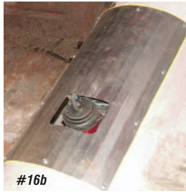
Photo #16a & 16b: With the transmission properly mounted, the new tunnel panel can be reinstalled. We elected to screw ours in place to make future access to the top of the transmission a snap.
