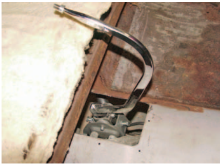
Photo #3: In order to install a floor shifter in a '55-'57 it is necessary to cut a hole in the floor. Sometimes you are lucky enough to have a hole that was cut neatly, but many times it looks like someone did it with a chain saw!
