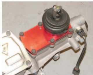
Photo #5: The Tremec transmission is a "top-loader" type transmission with the shifter base protruding out the top of the transmission case. This design gives far better shifting action than the old linkage type transmissions and is far more durable.
