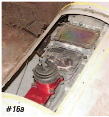
Photo #16a & 16b: With the transmission properly mounted, the new tunnel panel can be reinstalled. We elected to screw ours in place to make future access to the top of the transmission a snap.
