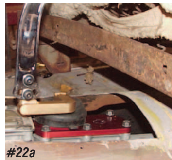
Photo #22a & 22b: With the offset shifter base, the curved shifter arm can be installed straight up giving plenty of clearance between the shifter arm and the seat with the seat in the reward position. If the seat is going to be moved forward you will want to install the arm in the forward hole. Photo (b) shows the shifter in 2nd gear with plenty of clearance between the shifter arm and the seat with the seat adjusted forward.
