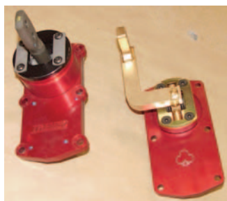
Photo #19: If a bench is going to be used and will be adjusted forward, the offset shifter base P/N 08-401 must be installed to clear the bench seat. The offset shifter base is a direct replacement for the shifter base that comes with the transmission. The shifter base is offset to the left 2" and forward 2-3/4". Curved shifter arm P/N 08-402 works great with this base as well.
