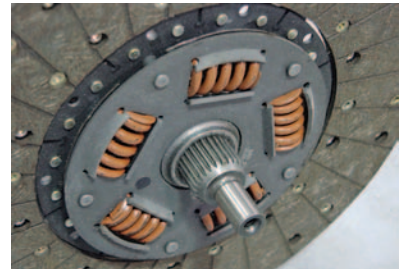
Photo #7: The input shaft (front) on a Tremec transmission has 26 splines. Make sure to get a clutch disc that matches the splines correctly.
