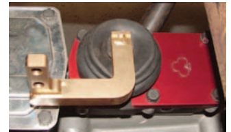
Photo #21: With the offset shifter base in place, transfer the rubber boot from the stock shifter base to the offset shifter base.
