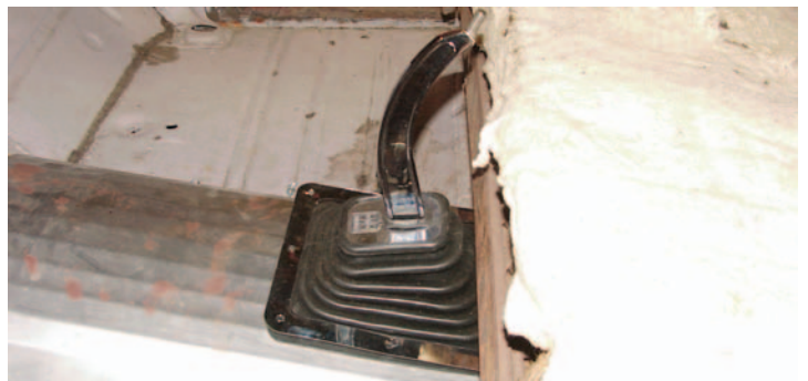
Photo #23: With the shifter base and arm installed, the shifter boot can be installed. The large HURST shifter boot P/N 208-09 works perfectly with the McLeod shifter.
