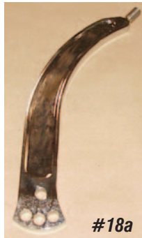
Photo #18a, 18b & 18c: The curved shifter arm P/N 08-402 attaches to the shifter with two 3/8" bolts. For a stock bench seat that will remain adjusted to the rear, install the shifter arm using the front lower hole. This will lean the arm forward and clear the bench seat. There are four mounting holes in the shifter arm allowing for several different shifter arm angles.
