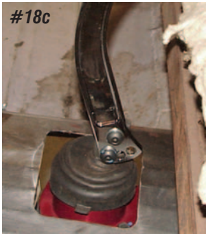
Photo #18a, 18b & 18c: The curved shifter arm P/N 08-402 attaches to the shifter with two 3/8" bolts. For a stock bench seat that will remain adjusted to the rear, install the shifter arm using the front lower hole. This will lean the arm forward and clear the bench seat. There are four mounting holes in the shifter arm allowing for several different shifter arm angles.
