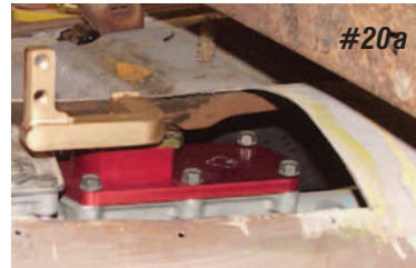
Photo #20a & 20b: The offset shifter base bolts to the top of the transmission using the six bolts that mounted the stock shifter base. Photo (a) shows the seat adjusted all the way to the rear, photo (b) shows the seat adjusted all the way to the front.
