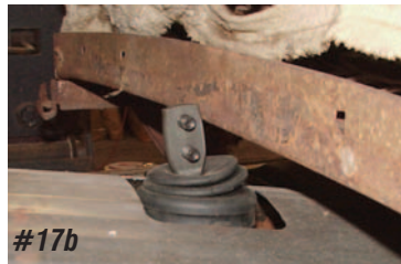
Photo #17a & 17b: If the bench seat is going to be used and remain in the rear-most adjustment position, the shifter that comes with the Tremec transmission can be used without adding an offset arm.
