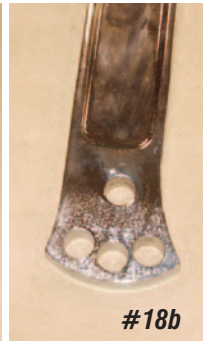
Photo #18a, 18b & 18c: The curved shifter arm P/N 08-402 attaches to the shifter with two 3/8" bolts. For a stock bench seat that will remain adjusted to the rear, install the shifter arm using the front lower hole. This will lean the arm forward and clear the bench seat. There are four mounting holes in the shifter arm allowing for several different shifter arm angles.
