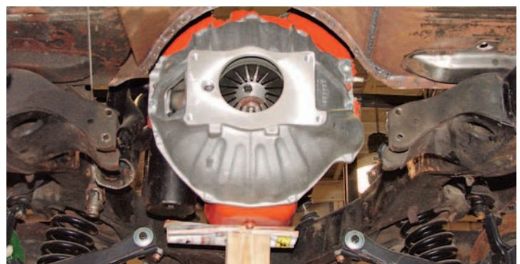
Photo #8: Our engine is going to be side mounted so the rear bell housing mounts can be eliminated. Install the new aluminum bellhousing P/N 08-23 .
