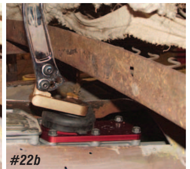
Photo #22a & 22b: With the offset shifter base, the curved shifter arm can be installed straight up giving plenty of clearance between the shifter arm and the seat with the seat in the reward position. If the seat is going to be moved forward you will want to install the arm in the forward hole. Photo (b) shows the shifter in 2nd gear with plenty of clearance between the shifter arm and the seat with the seat adjusted forward.
