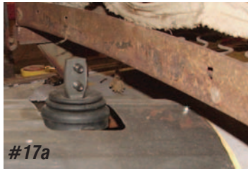
Photo #17a & 17b: If the bench seat is going to be used and remain in the rear-most adjustment position, the shifter that comes with the Tremec transmission can be used without adding an offset arm.
