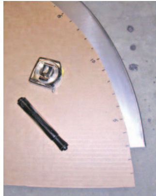
Photo #15: Raise the cheek template up into the opening in the trunk floor with the inch markings on the inboard side. Use C-clamps to hold the template to the frame. The center line of the template
