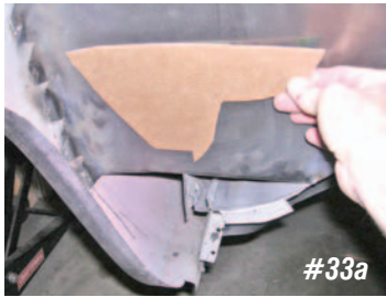
Photo #33a & 33b: At the front of the band there will be a gap between the band, the passenger compartment floor, and the rear quarter panel. A cardboard template was cut to fit the gap. The template was used to cut a patch panel out of a piece of 18 gauge sheet metal. The metal was tack welded into place, then welded solid with a continuous bead. The edge of the patch along the quarter panel will be sealed with autobody sealant, as will the band.
