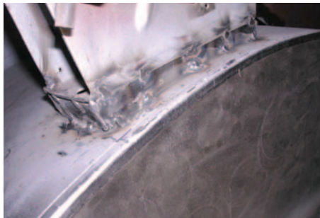
Photo #34: A pedestal was constructed to support the trunk hinge box and to strengthen the tub. The sides of the pedestal extend the walls of the hinge box down to the band. Paper templates were used to create the four sides. The templates were transferred to 18 gauge sheet metal and the pedestal sides were tack welded to both the hinge box and the band.
