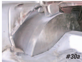
Photo #30a & 30b: The underside of the trunk floor along the cut lines was cleaned to bare metal and the tub was lowered into place one final time. When the fit was satisfactory the tub was tack welded to the trunk floor from underneath. The band was tack welded to the baffle from above.
