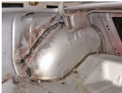
Photo #1: The trunk area of this car was in sad shape. The rear section of the original inner wheel tub had rusted away from the inner trunk wall. The rusty gap was over an inch wide and had been filled in by gobs
