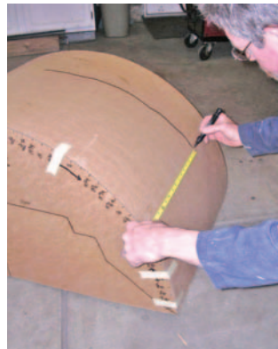
Photo #18: Remove the cheek template from the car. Use masking tape to attach the band template to the cheek template. Transfer the recorded measurements to the band and connect them to mark a cut line along the band. In order to make trial fitting of the tub template easier, we cut the band about one quarter inch short of this line.
