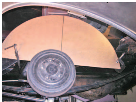
Photo #15: Raise the cheek template up into the opening in the trunk floor with the inch markings on the inboard side. Use C-clamps to hold the template to the frame. The center line of the template
