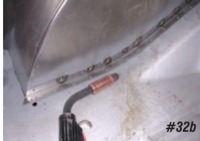
Photo #32a & 32b: The portion of the cheek template that was cut away and saved became a trunk floor contour guide for making a flange. The flange will help strengthen the joint between the floor
