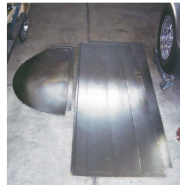
Photo #3: With the rear of the car up on jack stands, remove both rear wheels and the gas tank. Before cutting any sheet metal away, mark the inside of the outer quarter panel along the lower edge of the wheelhouse seal. The new wheel tub must meet the quarter panel near this line. Also mark the location and depth of the window dimple in the front wheelhouse section. This dimple allows necessary clearance for the rear corner of the rear quarter window.
