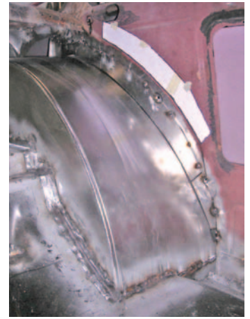
Photo #35: The inner quarter panel was then rebuilt. This panel consists mostly of flat sheet metal. Paper templates were made and metal patches were cut out of 18 gauge sheet metal. One of the templates is shown taped to the quarter panel just above its patch. These patches were tack welded into place on the quarter panel. Once tack welded into place they could be adjusted, tack welded to each other, and tack welded to the band. The patch at the peak of the band was welded to the new baffle. The level of finish for these welds is a matter of personal preference. These will be covered by upholstered side panels so perfect finish work is not needed.
