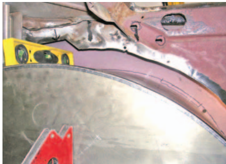
Photo #30a & 30b: The underside of the trunk floor along the cut lines was cleaned to bare metal and the tub was lowered into place one final time. When the fit was satisfactory the tub was tack welded to the trunk floor from underneath. The band was tack welded to the baffle from above.
