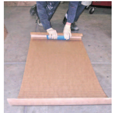
Photo #18: Remove the cheek template from the car. Use masking tape to attach the band template to the cheek template. Transfer the recorded measurements to the band and connect them to mark a cut line along the band. In order to make trial fitting of the tub template easier, we cut the band about one quarter inch short of this line.
