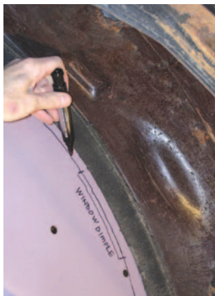
Photo #3: With the rear of the car up on jack stands, remove both rear wheels and the gas tank. Before cutting any sheet metal away, mark the inside of the outer quarter panel along the lower edge of the wheelhouse seal. The new wheel tub must meet the quarter panel near this line. Also mark the location and depth of the window dimple in the front wheelhouse section. This dimple allows necessary clearance for the rear corner of the rear quarter window.
