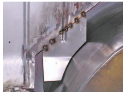
Photo #36: The repair of the inner trunk wall was more complicated since patch panels are not available for sedan body styles. The end of the fourth bead was compromised by rust and had to be cut away. We began by
