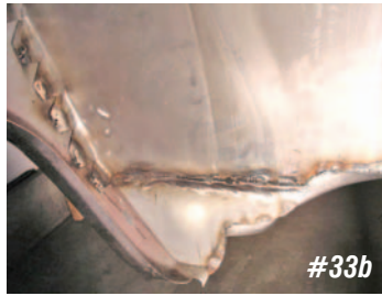
Photo #33a & 33b: At the front of the band there will be a gap between the band, the passenger compartment floor, and the rear quarter panel. A cardboard template was cut to fit the gap. The template was used to cut a patch panel out of a piece of 18 gauge sheet metal. The metal was tack welded into place, then welded solid with a continuous bead. The edge of the patch along the quarter panel will be sealed with autobody sealant, as will the band.
