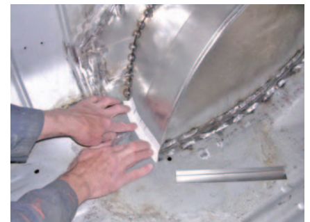
Photo #37: With the trunk wall and inner quarter repaired, flanges should be made to attach the front and rear edges of the band to the floor. Shown here is a paper template that was used as guide to make the cuts and notches on the flange material. Holes were punched
