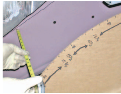
Photo #16: Measure from the cheek template to the inside of the quarter panel at every inch mark around the circumference. Keep the tape measure perpendicular to the cheek template and parallel to the ground.
