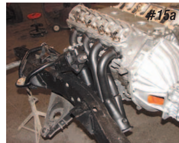
Photos #15a & #15b: Headers for the LS1 P/N 24-137 are available painted black or silver ceramic coated These headers will work with a stock steering box, 605, 670 power steering box or a CCI rack and pinion unit. The headers will not work with manual clutch linkage, so if a manual transmission is going to be used, a hydraulic clutch system must be installed. Refer to October 2006 Classic Chevy for complete instructions.
