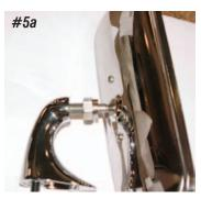
Photo #5a & 5b & 5c: The mirror bracket has 5/16"-18 mirror mounting threads so a standard mirror or a Day/-Night mirror or the Eckler's Classic Chevy aftermarket mirror mounting adaptor can
