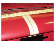
**Photo #2:** The mirror bracket can be mounted anywhere on the dashboard. On our 1955, we choose to mount the bracket center of the dashboard and close to the front edge of the dashboard. On a
