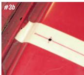
Photo #3a & 3b: We marked the center of our dashboard and measured back from the front edge 1-1/4". We will drill a 1/4" for the mounting stud on the mirror bracket. Use a sharp drill bit at a slow speed.
