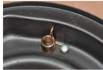
Photo #9: The new spring is held to the bucket with a #8 sheet metal screw, also supplied.
