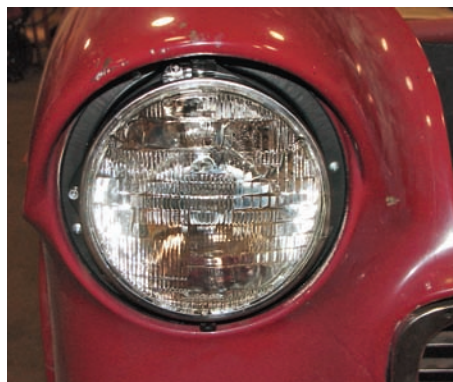
Photo #16a & 16b: The trim ring for the headlight is held to the sub bucket with three small sheet metal screws. Key the headlight and sub bucket assembly into the new adjuster screws and snap the spring into the hole in the ring using needle nose pliers.
