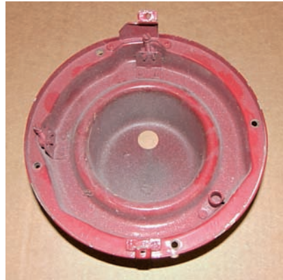
Photo #1: The bucket has two adjuster screws and a coil spring that attaches to the sub bucket both to hold it in place and for adjustment. Many times the nylon blocks on the adjusters strip out or break off and the hook on the spring will break.
