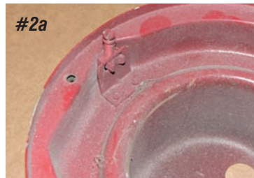
Photo #2a & 2b: The adjuster blocks are held to the bucket with a bracket that is riveted in place, while the spring is riveted directly to the bucket.
