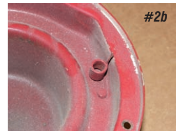
Photo #2a & 2b: The adjuster blocks are held to the bucket with a bracket that is riveted in place, while the spring is riveted directly to the bucket.
