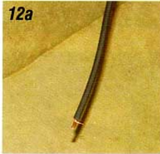
Photo #12a & 12b: Our project car already had the Raingear wiper system installed, so all we had to do was connect the brown wire from the washer pump to the brown wire on the Raingear wiper switch. To activate the windshield washers all you have to do is push the wiper switch button.
