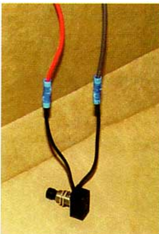
Photo #12a & 12b: Our project car already had the Raingear wiper system installed, so all we had to do was connect the brown wire from the washer pump to the brown wire on the Raingear wiper switch. To activate the windshield washers all you have to do is push the wiper switch button.
