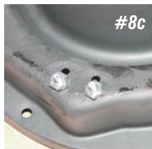
Photo #8a, 8b & 8c: The new adjuster brackets are attached to the bucket with two #10-32 X 3/4" machine screws, serrated washers and nuts supplied with the kit.
