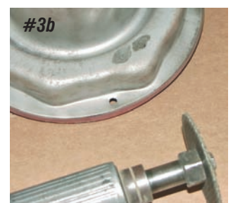
Photo #3a, 3b & 3c: Using a grinder from the backside of the bucket, grind the heads off the rivets that secure the adjuster blocks. Using a hammer and punch, drive the rivets out.
