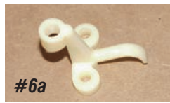
Photo #6a & 6b: The replacement adjuster brackets included in kit P/N 34-100 are made of nylon and attach to the headlight bucket using the supplied hardware. There is a tail on the replacement bracket that must be removed for this application. Using a pair of side cutters, remove half of the tail.
