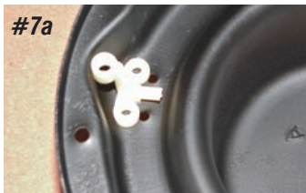
Photo #7a & 7b: New holes must be drilled for the new adjuster brackets. Using the original holes as a guide, line up the new bracket to the outside of the original holes and mark the bucket where the new holes need to be drilled. Drill two 3/16" holes for the new mounting hardware.
