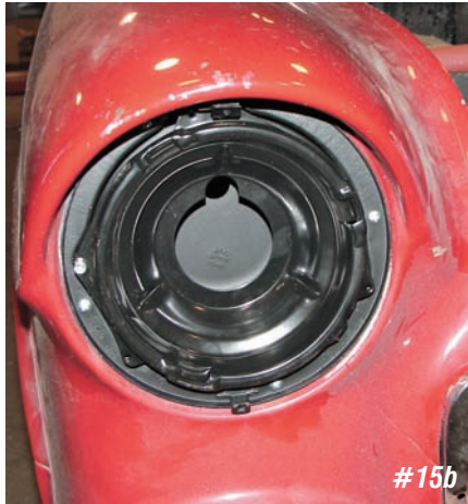
Photo #15a & 15b: Four #10 sheet metal screws are supplied to hold the bucket to the front fenders. These screws fit into the new J-nuts on the fenders.
