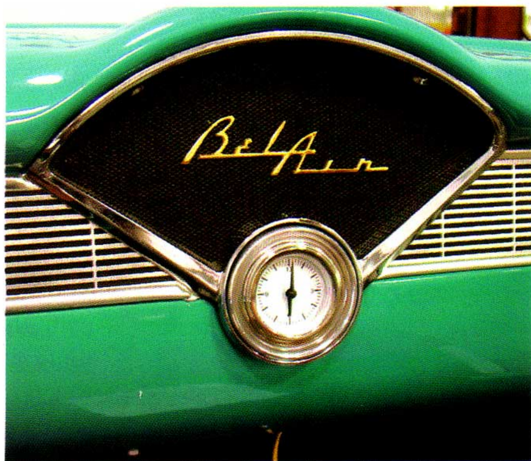
Photo #13: The speaker bezel and new clock may now be installed back into the dash.
