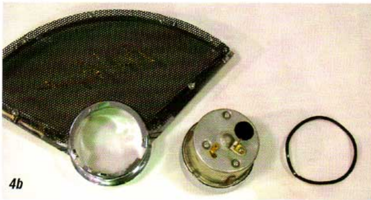
Photo #5: The new clock requires an adapter to fit the speaker bezel. This adapter is available in 3 different cut-styles and in polished or matte finish.
