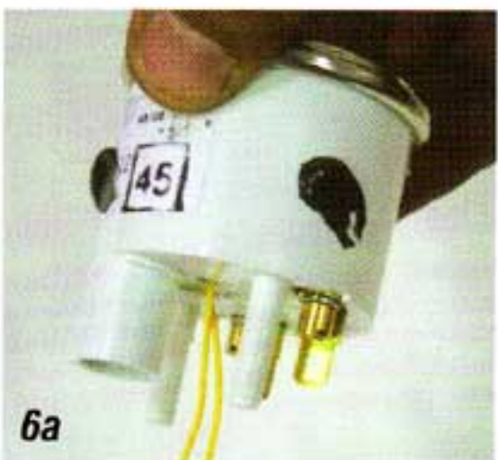
Photo #6a & 6b: The clock will glue into the adapter and the adapter and clock assembly will then glue into the speaker bezel. Put three or four dabs of silicone around the housing of the clock and install the clock into the adapter.
