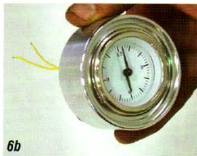
Photo #6a & 6b: The clock will glue into the adapter and the adapter and clock assembly will then glue into the speaker bezel. Put three or four dabs of silicone around the housing of the clock and install the clock into the adapter.
