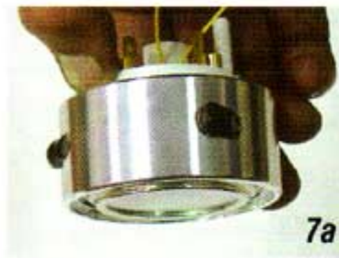
Photo #7a & 7b: Put three or four dabs of silicone around the outside of the clock adapter and install the adapter in the speaker bezel. Make sure the clock is oriented correctly and not crooked. Allow the silicone to dry for at least 30 minutes before installing the bezel back into the dash.
