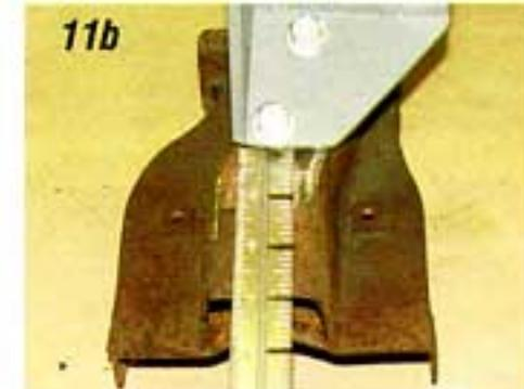
**Photo #11a & 11b:** On the 1957 pedal assembly both 3/8" holes must be drilled for the clutch master cylinder bracket. The rear edge of the bracket should be located 2-7/8" from the rear edge of the pedal assembly. The original support rods from the pedal assembly to cowl will no longer be used.
