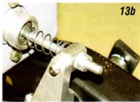
**Photo #13a & 13b:** The master cylinder is equipped with a threaded pushrod. The 3" long spring provided should be installed onto the pushrod shaft first. Screw the coupler onto the shaft to connect the master cylinder pushrod to the clutch pedal arm. Make sure the flat side on the coupler is facing away from the master cylinder.
