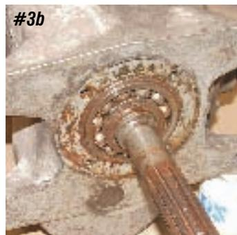
**Photo #3a & 3b:** To remove the bearing retainer, first bend the tabs back on the bolt retaining plates and remove the four bolts. Using a plastic mallet, tap on the neck of the retainer and the retainer will break free from the transmission.
