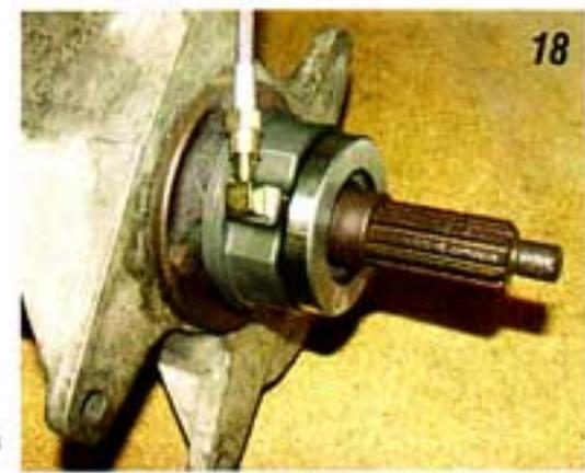
**Photo #19:** The release bearing is adjustable in length so that it can be used with a diaphragm or three finger type pressure plate. A set collar on the release bearing may be adjusted in or out to set the proper clearance between the release bearing and pressure plate.
