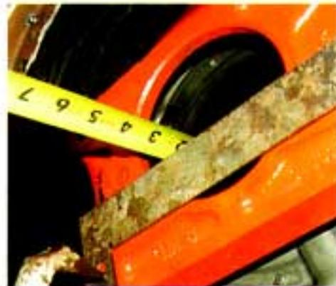
**Photo #23:** Next measure the distance from the face of the bellhousing to the fingers on the pressure plate. Our project car had a measurement of 2-7/8". By subtracting 2-7/8" from the 3" measurement we find that we have 1/8" (.125")
