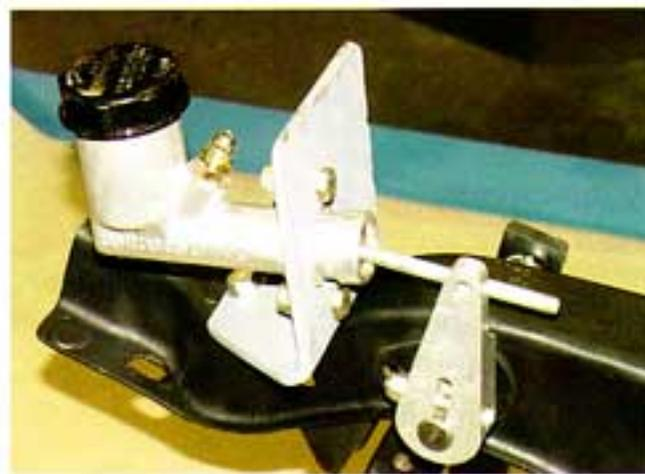
**Photo #12:** The clutch master cylinder bolts to the master cylinder bracket with two 5/16" X 1-1/4" bolts with lock nuts.
