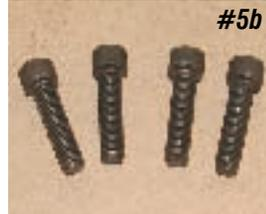
**Photo #5a & 5b & 5c:** Before installing the hydraulic release bearing, the manufacturer recommends putting a thin coat of silicone sealer on the face of the bearing and not using the stock bearing retainer gasket. Using the supplied socket head bolts, bolt the retainer to the front of the
