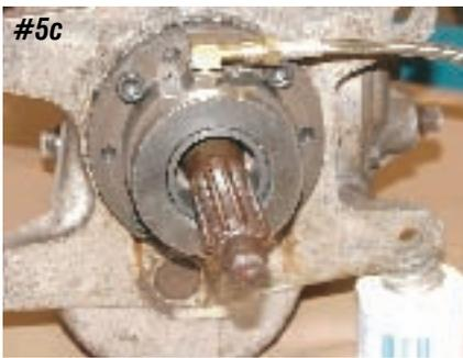
transmission and torque the bolts to 18 ft/lbs.
