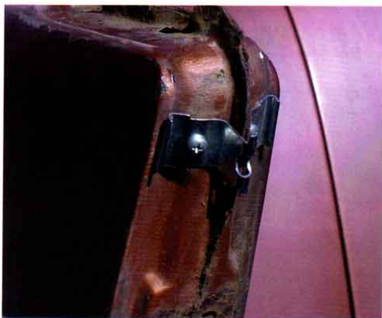
Photo #7: The fin molding is held to the rear of the quarter panel on each side with clips #34-161. This clip is held to the body with two sheet metal screws provided.
