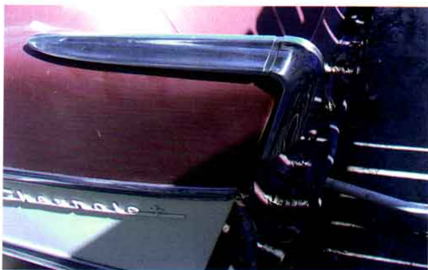
Photo #9: To install the two moldings on the car, first start with the fin molding, slide the fin molding half way down onto the clip on the rear of the quarter panel. Then couple the crown molding to the fin molding and work the two moldings together as you push down and forward. Some gentle bumping with the palm of your hand should force the moldings into place.
