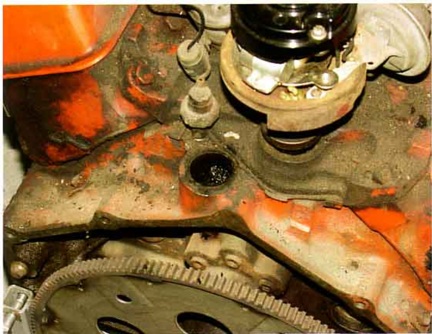
Photo #2: Remove the 7/16" bolt from the center of the road draft tube. The road draft tube has a tab that holds the spark plug wires in place on the passenger side. After removing the tube, pull the wires out of the tube bracket and make sure they are pulled back away from the exhaust manifold.
