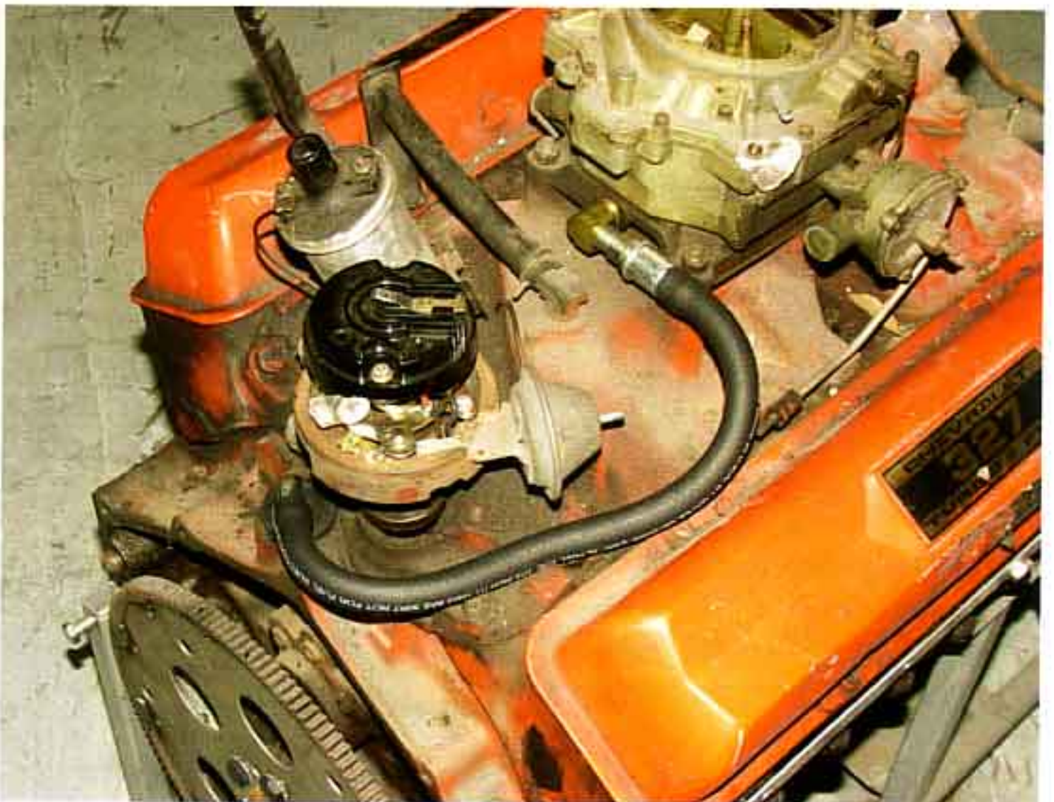
Photo #6: The kit includes 12" of 7/16" vacuum hose. Connect one end of the hose to the PCV valve and the other to the 90-degree elbow at the carburetor. With the crankcase properly vented, you will no longer have an oil mess under your car and the job of keeping the engine compartment cleaner just got easier! Good Luck!
