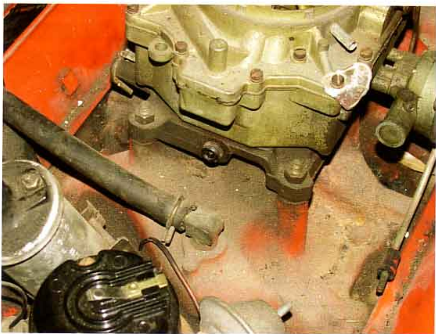
Photo #4: On the carburetor baseplate at the rear there is a 1/4" pipe plug that will need to be removed. The new valve requires full intake vacuum to work properly.
