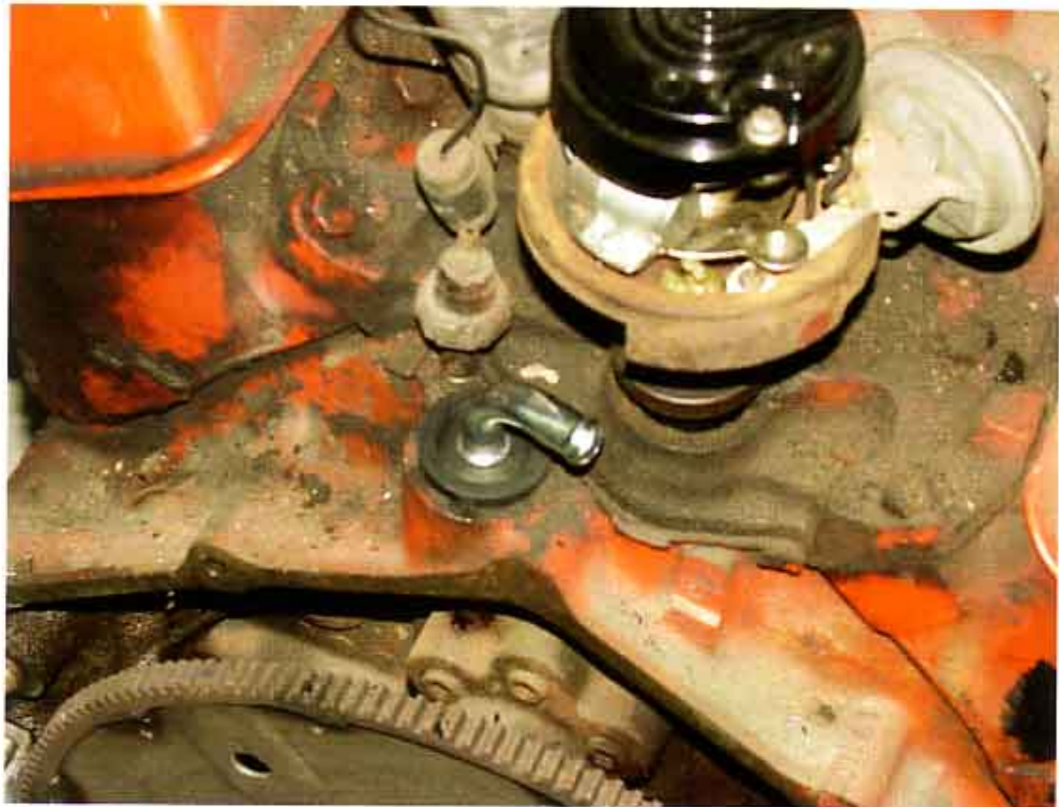
Photo #3: The hole in the block where the tube was just removed is connected to a vapor can under the intake manifold. This is where the PCV valve will draw the oil vapors from the engine. Install the large grommet and 90-degree elbow into this hole.
