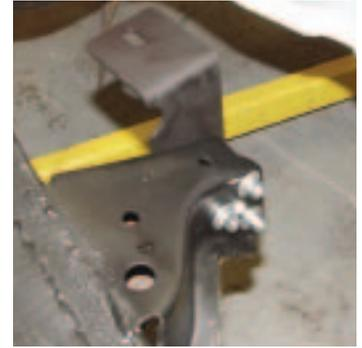
**Photo #6a & 6b:** The lower half of the new transmission supports bolt to the front of the original frame horns with three 3/8" X 3-1/4" bolts, flat washers, lock washers and nuts. There is a cut-out on the drivers side lower bracket to allow the front emergency brake cable to pass by.
