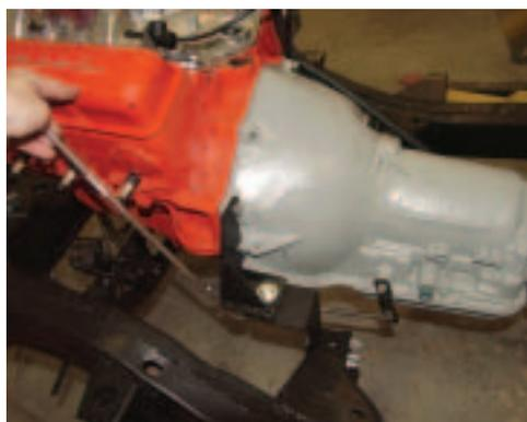
**Photo #28:** Shifter linkage P/N 19-19 connects the transmission to the stock or aftermarket steering column.
