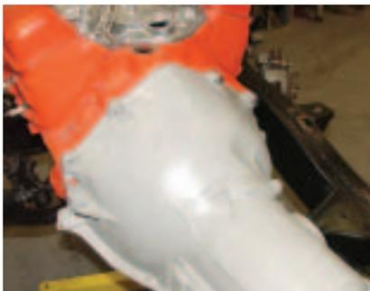
**Photo #9:** With the bellhousing bolted to the engine, bolt the torque converter to the flexplate using the supplied metric bolts.
