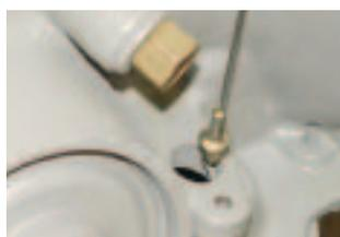
**Photo #19:** The kickdown/TVI cable **P/N 19-64** is the same as a TVI cable for a TH700-R4. The cable connects to a hook inside the kickdown cavity on the right hand side of the transmission.
