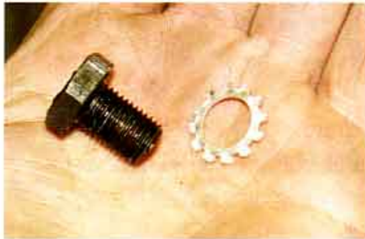
Photo #3: The flywheel is held to the crankshaft with five 7/16" X 11/16" fine thread bolts with serrated lock washers P/N 19-62. Torque these bolts to 45 ft/lbs.
