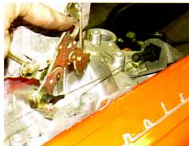
Photo #24a & 24b: Connect the plastic clip from the kickdown cable to the kickdown pin on the carburetor. Adjust the cable using the barrel clamp so that when the carburetor is at full throttle the cable is pulled tight.
