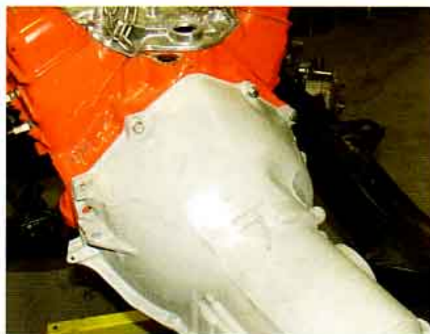
Photo #5: Raise the transmission and attach to the engine with the top two bellhousing-to-engine-block bolts and lock washers.
