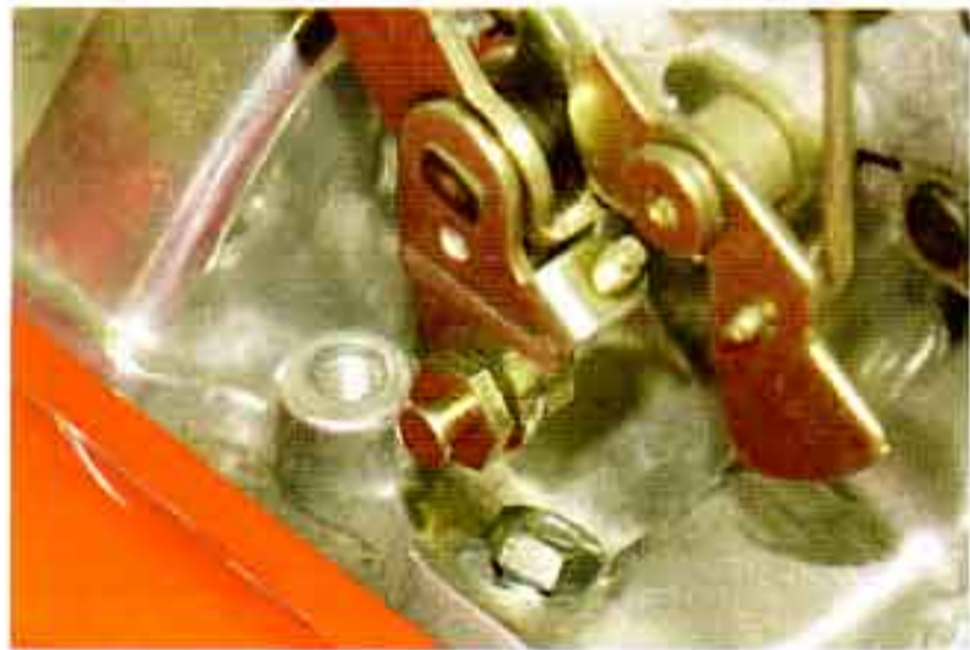
Photo #23: The kickdown cable pin P/N 19-66 bolts to the lower throttle arm.
