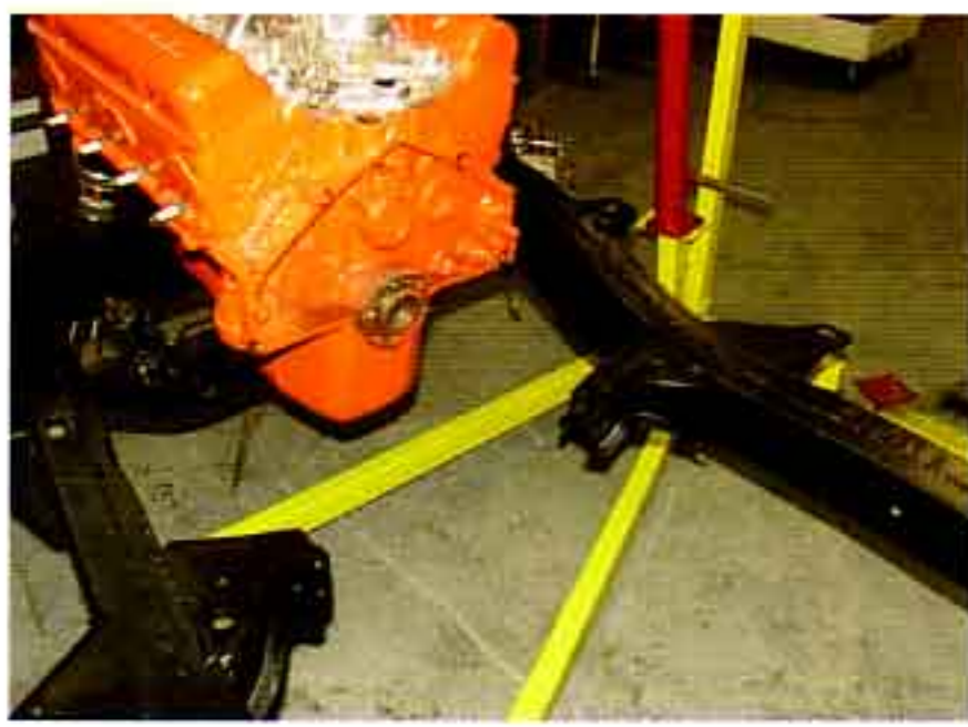
Photo #1: The original engine was mounted to the main crossmember with rubber grommets and studs. The rear of the engine was held in place with mounts from the bellhousing to the frame horns.
