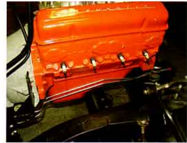
Photo #26a & 26b: The transmission cooler lines P/N 19-24 are designed to route around the dipstick and tube, feed around the starter and connect to the stock radiator in the V-8 position. Other lines, P/N 19-41 are available for cars with radiators in the 6-cylinder position.
