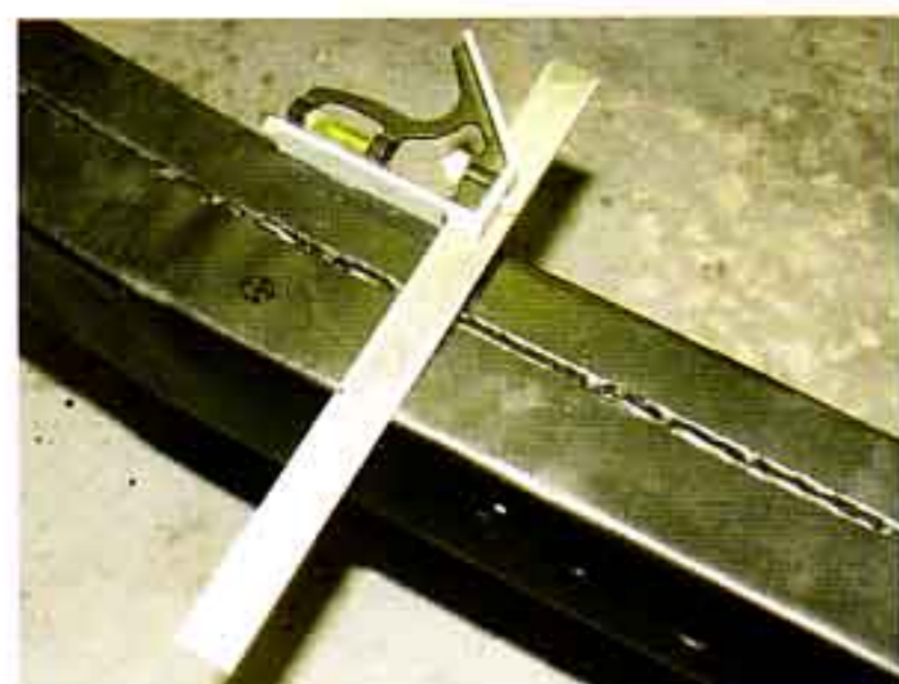
Photo #15: Remove the crossmember and elbow mounting brackets. Using a square, mark the outside of the frame and drill all four 3/8" elbow mounting bracket holes.
