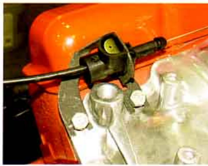
Photo #21a & 21b: The kickdown bracket P/N 19-23 mounts to the two rear intake bolts on the drivers side of the engine.
