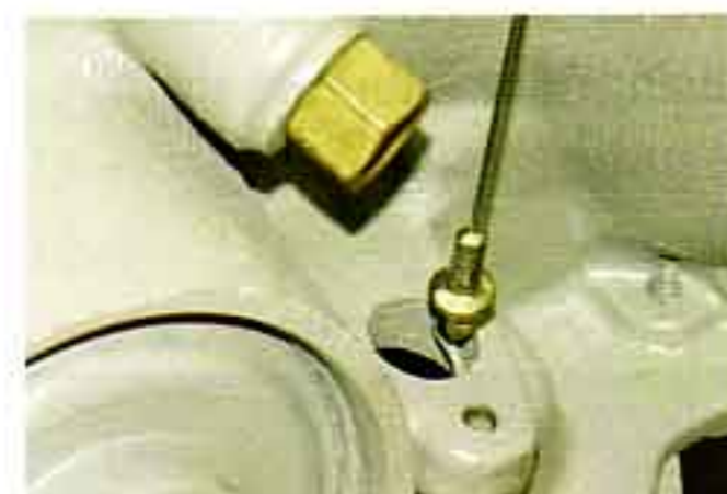
Photo #19: The kickdown/TVI cable P/N 19-64 is the same as a TVI cable for a TH700-R4. The cable connects to a hook inside the kickdown cavity on the right hand side of the transmission.
