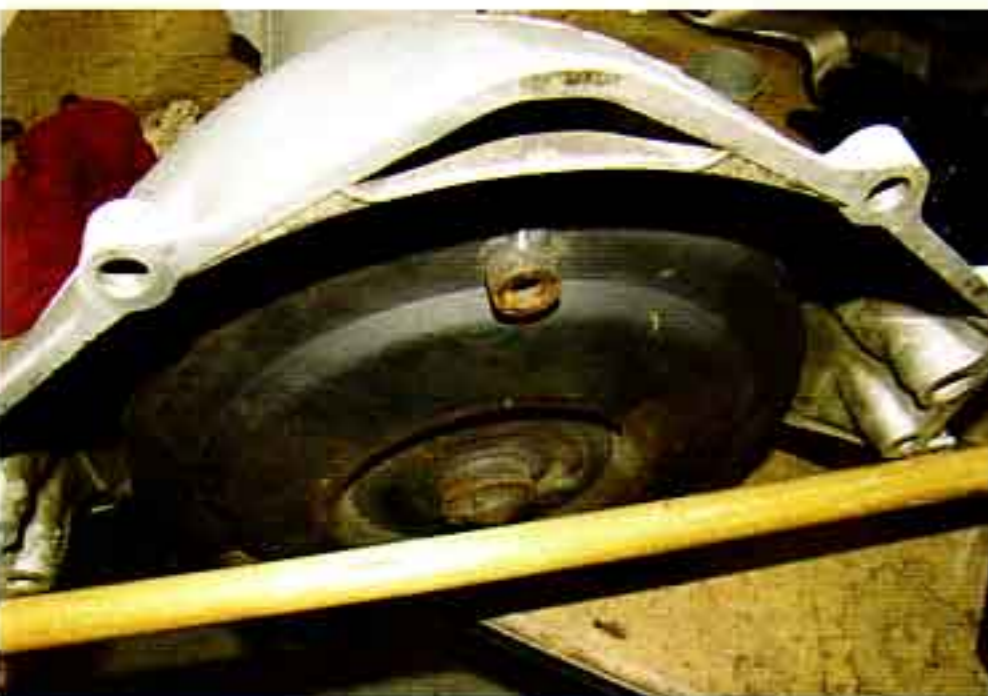
Photo #4: Make sure the torque converter is installed all the way into the front of the transmission. If the torque converter is not installed all the way and the transmission is
