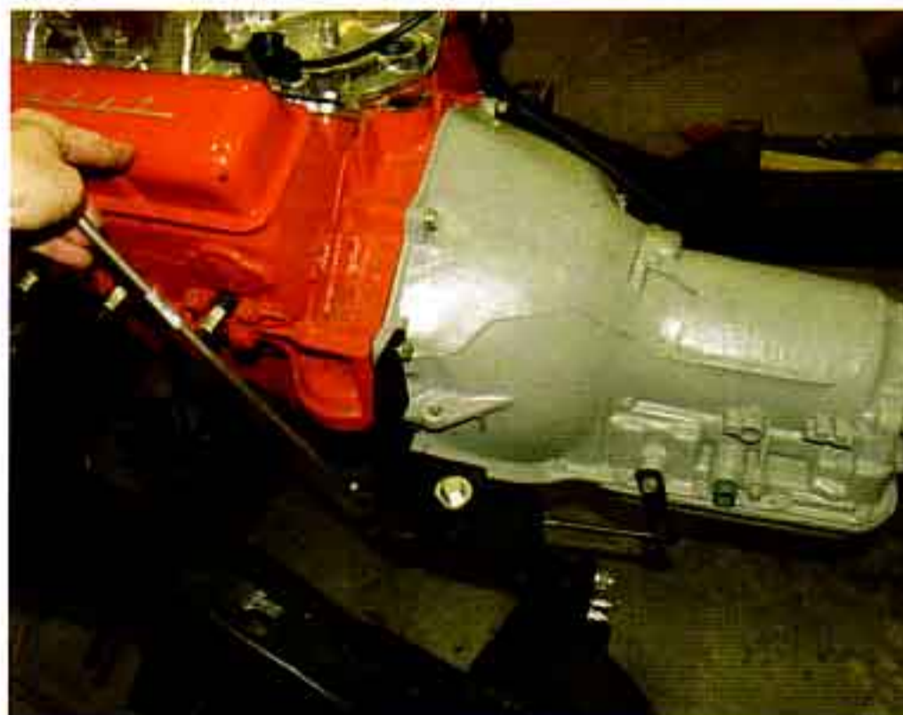
Photo #28: Shifter linkage P/N 19-19 connects the transmission to the stock or aftermarket steering column.
