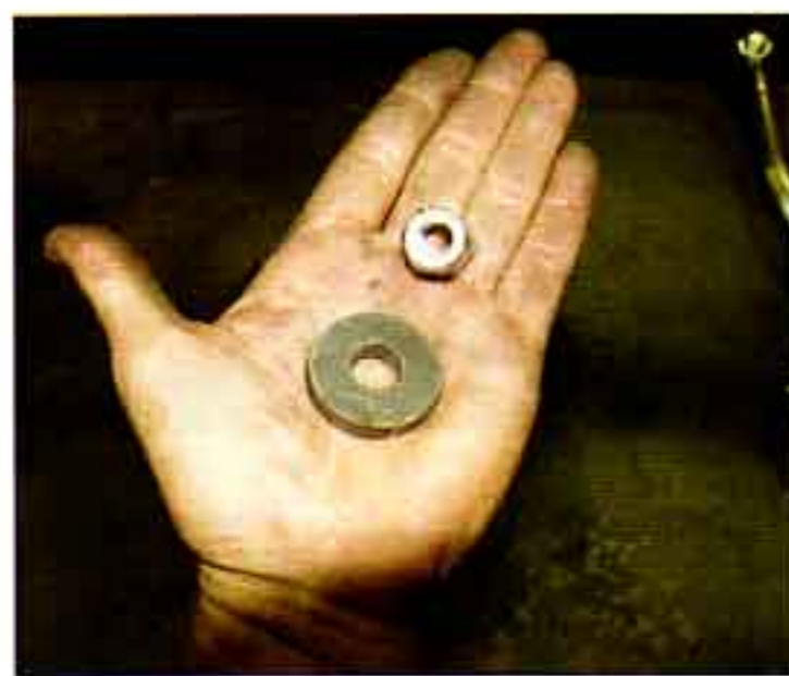
Photo #13a & 13b: The transmission crossmember bolts to the elbow brackets with a 1/2" X 3" bolt. There is a flat washer on the top of the crossmember and a heavy 1/4" thick flat washer and lock nut on the bottom of the elbow bracket.
