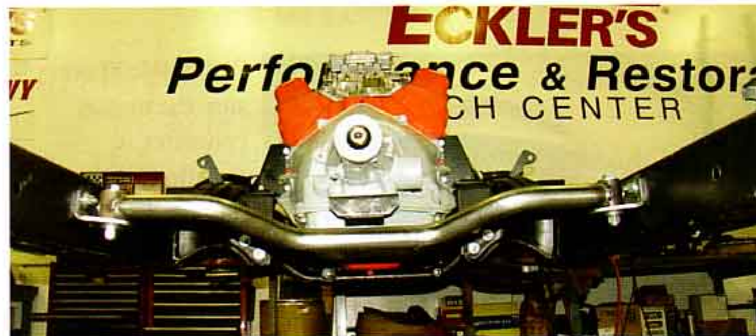
Photo #18: The crossmember has plenty of offset to allow any size or type of exhaust system to pass underneath.
