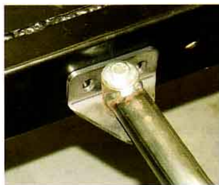
Photo #13a & 13b: The transmission crossmember bolts to the elbow brackets with a 1/2" X 3" bolt. There is a flat washer on the top of the crossmember and a heavy 1/4" thick flat washer and lock nut on the bottom of the elbow bracket.
