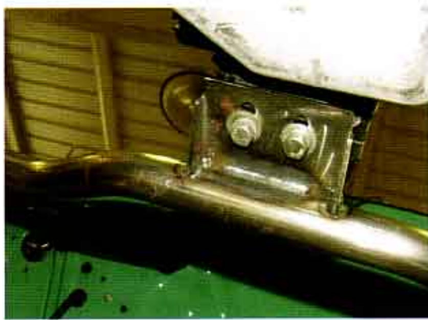
Photo #12: The outer elbow brackets for the transmission crossmember bolt to the frame using two 3/8" carriage bolts. The brackets have a mounting slot for the crossmember to allow for any variations in the frame width.
