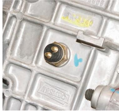
**Photo 17:** There are several electrical senders on the Tremec transmission case. The upper forward 2-pin sender on the driver's side of the transmission is the sender for the back-up lights. To connect the back-up lights to the sender, connect one of the pins of the sender to a key on fused
