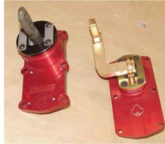
**Photo 4:** If the stock front bench seat is going to be used and adjusted forward, or if you prefer the shifter to be in a position similar to the 3 or 4-speed transmission, the McLeod offset shifter P/N 08-401 will need to be used. This shifter offsets the shifter arm 2" to the left (driver's side) and 2-3/4" forward. The McLeod shifter bolts in place of the stock Tremec shifter.
