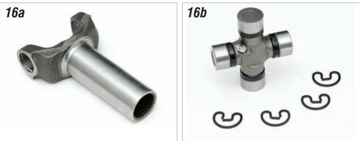
**Photos 16a & 16b:** The Tremec transmission uses a Ford C-6 automatic driveshaft slip yoke P/N 19-299. P/N 19-300 U-joint will adapt the Ford style yoke to the Chevy driveshaft.
