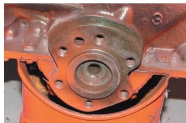
**Photo 6:** A new brass pilot bushing is included with the clutch and pressure plate kit. The bushing is installed in the rear crank hub to support the input shaft of the transmission on the flywheel side of the clutch disc. The bushing is driven in flush with the hub of the crankshaft. Grease the inner bore of the pilot bushing with chassis grease.
