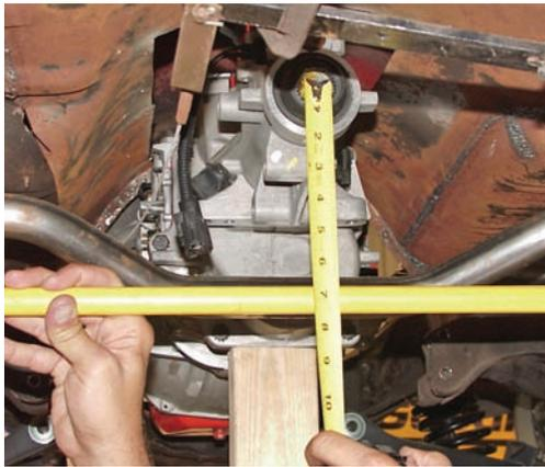
**Photo 11:** When mounting the transmission crossmember to the frame rails, the output shaft of the transmission must measure  $6-1/2"$  from the center to the bottom of the frame rails. The brackets for the
