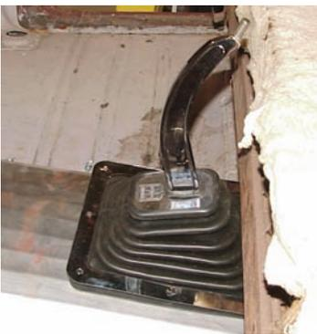
**Photo 15:** The large Hurst shifter boot P/N 208-09 works great with the McLeod shifter. The boot is held to the floor with six #6 sheet metal screws. This boot is not included in the Tremec installation kit. A white P/N 08-404 or black P/N 08-405 5-speed shifter ball is available for the McLeod shifter.
