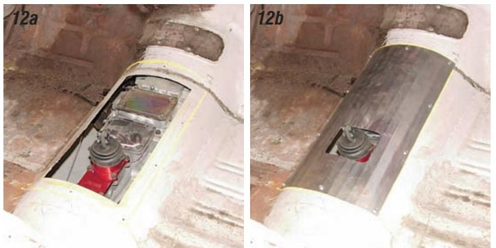
**Photos 12a & 12b:** The Tremec transmission case is fairly large and will make contact with the stock transmission hump. Tunnel **P/N 31-350** is a 16 gauge panel that can be installed in place of the stock hump to provide enough clearance for the Tremec case. The panel can be welded in or held in with tech screws. The stock carpet will still work perfectly.
