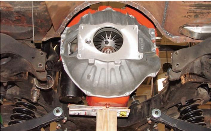
**Photo 9:** You may install the Tremec using the stock cast iron bellhousing if you desire. The aluminum bellhousing **P/N 08-23** is a reproduction of the mid to late 60's GM bellhousing and can be used with side engine mounts only. The bellhousing bolts to the back of the engine with six supplied  $3/8"$  X  $1-1/4"$  bolts and lock washers.
