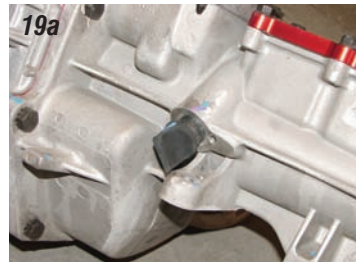
Photos 19a & 19b: On both sides of the tailshaft housing you will find two plugs. The plug on the passenger side is for an electrical speedometer. The rubber plug on the driver's side is for a mechanical speedometer cable. If an electrical speedometer is going to be used, install the supplied aluminum plug into the hole on the driver's side of the tailshaft housing. If a mechanical speedometer is going to be used then P/N 19-223 speedometer cable kit must be ordered. When ordering the speedometer cable kit, you will need to supply the rear tire height and rear end gear ratio.
