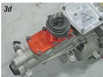
Photos 3a, 3b, 3c & 3d: The Tremec transmission P/N 08-400 includes the factory Tremec shifter. The shifter will be installed in the rear-most position when delivered. If bucket seats are going to be used, the stock Tremec shifter can be used and will remain in this position. If a stock bench seat is used and is adjusted all the way to the rear (or if buckets are used and adjusted forward), the shifter will need to be moved to the front mount position. The shifter is held to the transmission case with six metric bolts. Remove the six bolts and rotate the shifter 180 degrees so that it is oriented toward the front. Clean the base of the shifter, apply a small amount of gasket sealer to the shifter and bolt the shifter back in place. Torque the bolts to 21 ft/lbs. This shifter will keep the shifter arm in the center of the transmission and the center of the transmission hump, unlike the 3 or 4-speed shifters, which are mounted to the side of the transmission offsetting it closer to the driver.
