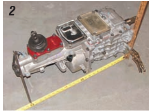
Photos 3a, 3b, 3c & 3d: The Tremec transmission P/N 08-400 includes the factory Tremec shifter. The shifter will be installed in the rear-most position when delivered. If bucket seats are going to be used, the stock Tremec shifter can be used and will remain in this position. If a stock bench seat is used and is adjusted all the way to the rear (or if buckets are used and adjusted forward), the shifter will need to be moved to the front mount position. The shifter is held to the transmission case with six metric bolts. Remove the six bolts and rotate the shifter 180 degrees so that it is oriented toward the front. Clean the base of the shifter, apply a small amount of gasket sealer to the shifter and bolt the shifter back in place. Torque the bolts to 21 ft/lbs. This shifter will keep the shifter arm in the center of the transmission and the center of the transmission hump, unlike the 3 or 4-speed shifters, which are mounted to the side of the transmission offsetting it closer to the driver.
