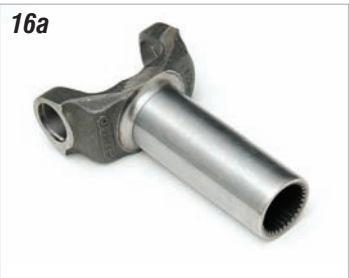
Photos 16a & 16b: The Tremec transmission uses a Ford C-6 automatic driveshaft slip yoke P/N 19-299. P/N 19-300 U-joint will adapt the Ford style yoke to the Chevy driveshaft.
