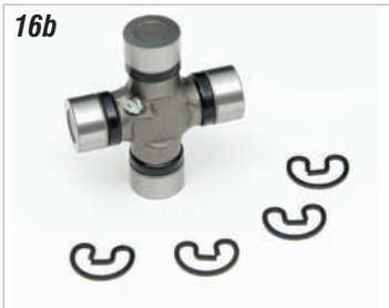
Photos 16a & 16b: The Tremec transmission uses a Ford C-6 automatic driveshaft slip yoke P/N 19-299. P/N 19-300 U-joint will adapt the Ford style yoke to the Chevy driveshaft.
