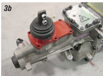
Photos 3a, 3b, 3c & 3d: The Tremec transmission P/N 08-400 includes the factory Tremec shifter. The shifter will be installed in the rear-most position when delivered. If bucket seats are going to be used, the stock Tremec shifter can be used and will remain in this position. If a stock bench seat is used and is adjusted all the way to the rear (or if buckets are used and adjusted forward), the shifter will need to be moved to the front mount position. The shifter is held to the transmission case with six metric bolts. Remove the six bolts and rotate the shifter 180 degrees so that it is oriented toward the front. Clean the base of the shifter, apply a small amount of gasket sealer to the shifter and bolt the shifter back in place. Torque the bolts to 21 ft/lbs. This shifter will keep the shifter arm in the center of the transmission and the center of the transmission hump, unlike the 3 or 4-speed shifters, which are mounted to the side of the transmission offsetting it closer to the driver.
