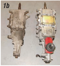
Photos 1a & 1b: The Tremec 5-speed transmission P/N 08-400 has the same bellhousing bolt pattern as the early model GM Muncie and Saginaw 3 and 4-speed transmissions.
