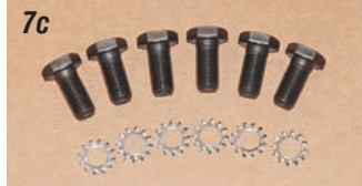
Photos 7a, 7b, 7c & 7d: The flywheel P/N 08-409 is for an internally balanced small block or big block engine and will accept a 10-1/2" or 11" clutch and pressure plate. The flywheel is held to the crankshaft with six 7/16" standard transmission flywheel bolts P/N 19-61 and serrated lock washers. Always use a small amount of thread locker on the flywheel and pressure plate bolts. Torque the flywheel bolts to 65 ft./lbs.
