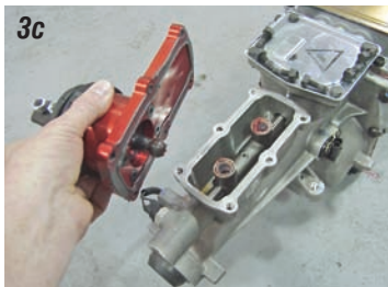
Photos 3a, 3b, 3c & 3d: The Tremec transmission P/N 08-400 includes the factory Tremec shifter. The shifter will be installed in the rear-most position when delivered. If bucket seats are going to be used, the stock Tremec shifter can be used and will remain in this position. If a stock bench seat is used and is adjusted all the way to the rear (or if buckets are used and adjusted forward), the shifter will need to be moved to the front mount position. The shifter is held to the transmission case with six metric bolts. Remove the six bolts and rotate the shifter 180 degrees so that it is oriented toward the front. Clean the base of the shifter, apply a small amount of gasket sealer to the shifter and bolt the shifter back in place. Torque the bolts to 21 ft/lbs. This shifter will keep the shifter arm in the center of the transmission and the center of the transmission hump, unlike the 3 or 4-speed shifters, which are mounted to the side of the transmission offsetting it closer to the driver.
