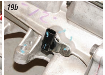
Photos 19a & 19b: On both sides of the tailshaft housing you will find two plugs. The plug on the passenger side is for an electrical speedometer. The rubber plug on the driver's side is for a mechanical speedometer cable. If an electrical speedometer is going to be used, install the supplied aluminum plug into the hole on the driver's side of the tailshaft housing. If a mechanical speedometer is going to be used then P/N 19-223 speedometer cable kit must be ordered. When ordering the speedometer cable kit, you will need to supply the rear tire height and rear end gear ratio.
