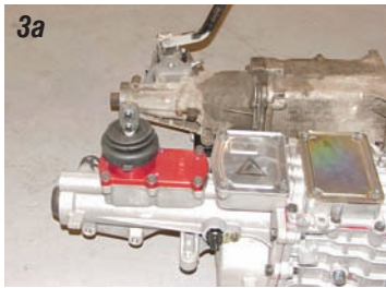
Photos 3a, 3b, 3c & 3d: The Tremec transmission P/N 08-400 includes the factory Tremec shifter. The shifter will be installed in the rear-most position when delivered. If bucket seats are going to be used, the stock Tremec shifter can be used and will remain in this position. If a stock bench seat is used and is adjusted all the way to the rear (or if buckets are used and adjusted forward), the shifter will need to be moved to the front mount position. The shifter is held to the transmission case with six metric bolts. Remove the six bolts and rotate the shifter 180 degrees so that it is oriented toward the front. Clean the base of the shifter, apply a small amount of gasket sealer to the shifter and bolt the shifter back in place. Torque the bolts to 21 ft/lbs. This shifter will keep the shifter arm in the center of the transmission and the center of the transmission hump, unlike the 3 or 4-speed shifters, which are mounted to the side of the transmission offsetting it closer to the driver.
