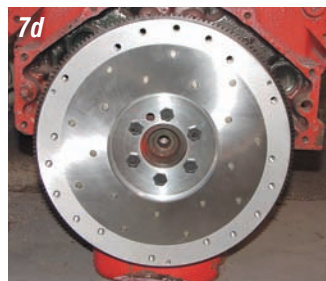
Photos 7a, 7b, 7c & 7d: The flywheel P/N 08-409 is for an internally balanced small block or big block engine and will accept a 10-1/2" or 11" clutch and pressure plate. The flywheel is held to the crankshaft with six 7/16" standard transmission flywheel bolts P/N 19-61 and serrated lock washers. Always use a small amount of thread locker on the flywheel and pressure plate bolts. Torque the flywheel bolts to 65 ft./lbs.
