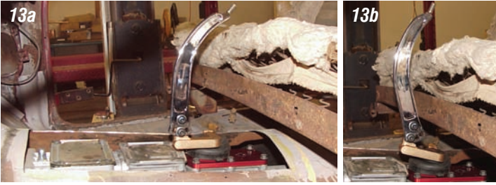
Photos 13a & 13b: When using the offset shifter P/N 08-401, there is plenty of room for the bench seat to be all the way forward or all the way back.
