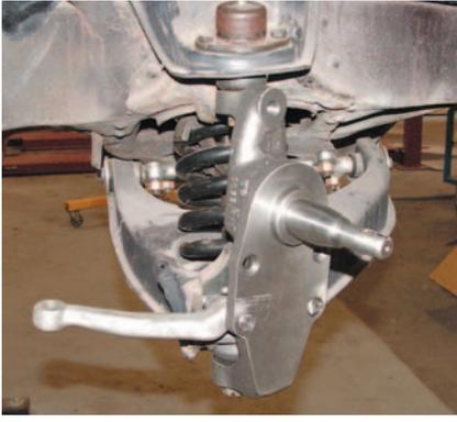
**Photo #7:** Install the new dropped spindles on the ball joint studs and secure with the ball joint nuts and new cotter pins. Install the coil springs and shocks. If you desire a 4" drop, this is the time to install 2" lowering coils P/N 21-133.
