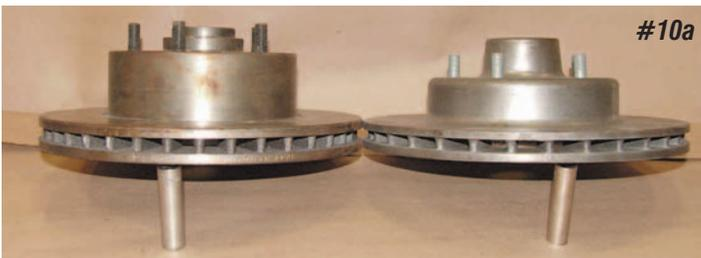
**Photos #10a & #10b:** Special rotor P/N 20-126 (provided in the dropped spindle brake kits) must be used with the dropped spindle kit. This rotor positions the wheels 1/4" inboard from the stock drum location and has the correct offset for the large GM caliper. This rotor uses the larger inner and outer wheel bearings
