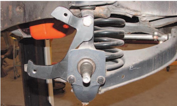
**Photo #2:** The disc brake bracket for the stock spindle bolts to the top of the spindle using the original large wheel cylinder mount and to the lower rear hole where the steering arm mounts. The new dropped spindles come with their own caliper brackets so the brackets above will not be used.
