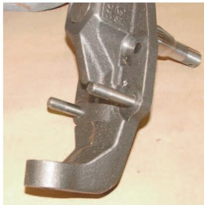
**Photo #5:** There are two 7/16" studs pressed into the dropped spindle P/N 21-103. These studs are to secure the steering arms that connect to the outer tie rod ends. The longer stud is oriented to the rear of the spindle.
