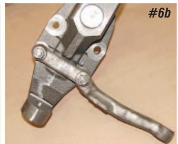
**Photos #6a & #6b:** The boss on the steering arm is thicker at the rear thus the need for the longer stud. The arm will be held to the spindle with 7/16" lock nuts supplied with the dropped spindles.
