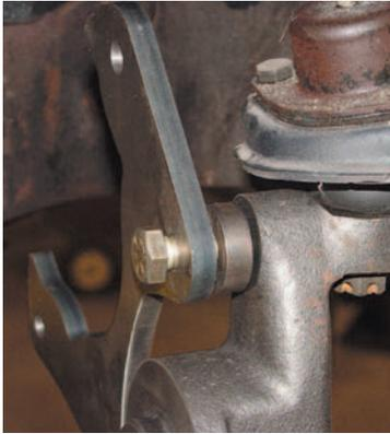
**Photo #8:** The disc brake bracket supplied with the dropped spindle kit is designed for the large GM caliper and is bolted directly to the dropped spindle. A 1/2" x 1-1/4" bolt secures the bracket to the top of the spindle using a supplied 3/8" spacer between the bracket and spindle. The bracket faces to the rear of the spindle.
