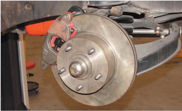
**Photo #1:** All Classic Chevy disc brake kits use large 11" GM rotors and the large GM calipers. Most other kits on the market use the smaller 10" S-10 pickup rotors and the small mid-sized car calipers. Any disc brake kit is better than an original drum brake system, but bigger is always better when you are talking about brakes. The S-10 rotors use a very small inner bearing as well which can be a weak point compared to the full-size car bearings used with our kits.
