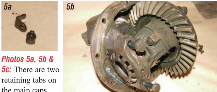
**Photos 5a, 5b & 5c:** There are two retaining tabs on the main caps that hold the side carrier adjusters in place. Remove the two 1/2" X 1/2" bolts that secure the retainers. Next, remove two main cap bolts, main caps and side adjusters.
