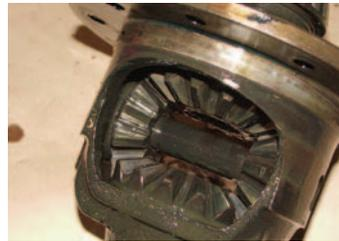
**Photo 8:** Shown is the weak point on the stock carrier: no thrust washer between the side gears or spider gears and the carrier is used.
