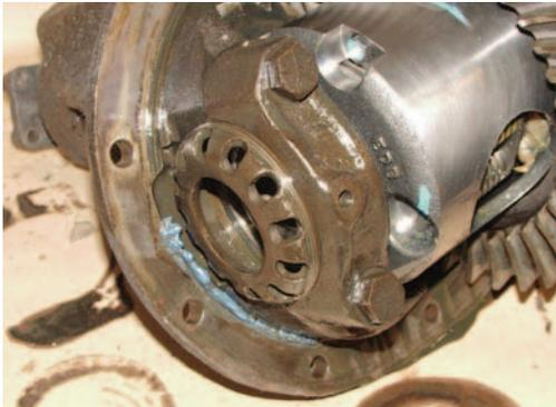
**Photo 12:** With the carrier in place, install the two main caps and side adjusters. Torque the main cap bolts to 70-75 ft/lbs.
