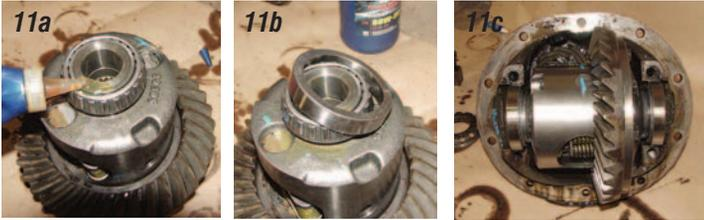
**Photos 11a, 11b & 11c:** Before installing the carrier into the center section, put plenty of gear lube on the new carrier bearings. Install new bearing races **P/N 21-116** on each side of the carrier and place the carrier in the center section.
