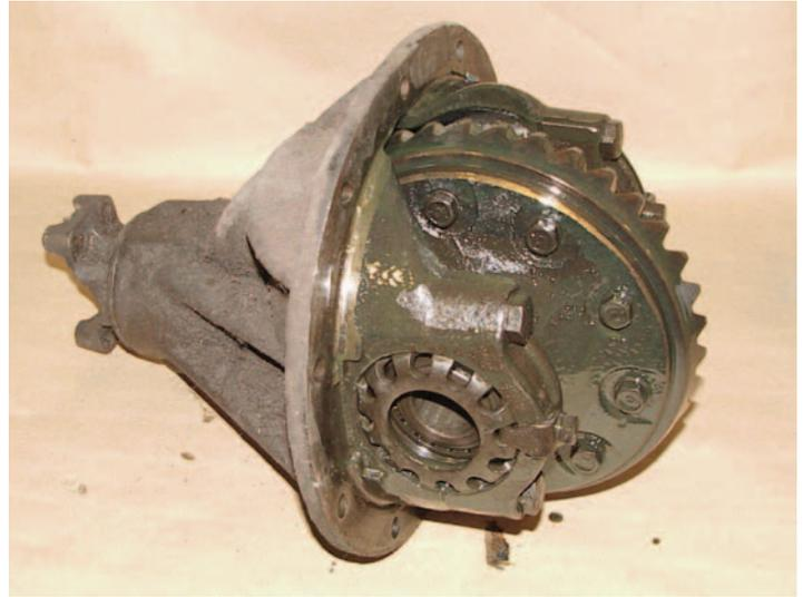
**Photo 1:** The 1955 through 1964 Chevy had a front loader type rear end with no removable rear end cover. The carrier is often referred to as the chunk, the pig, the pumpkin or the center section. This means the ring and pinion, carrier and case is removed from the front side of the rear end housing as a unit.
