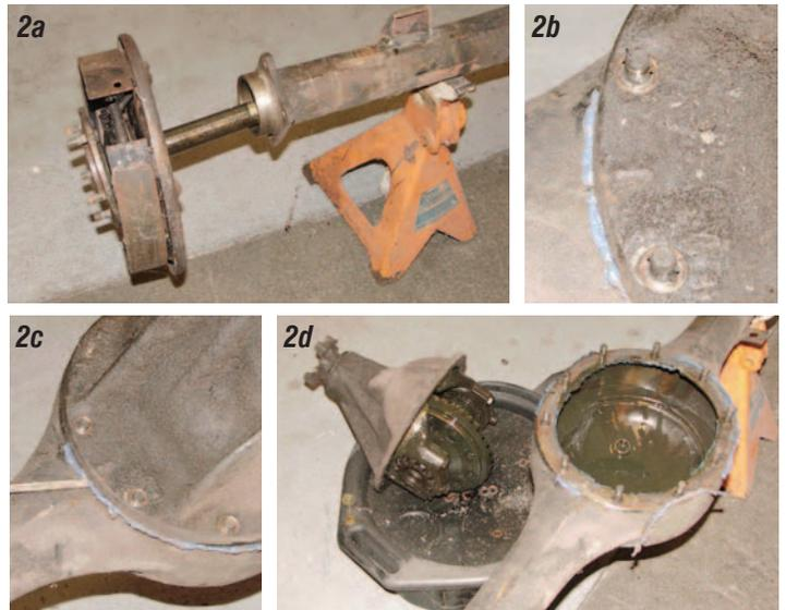
**Photos 2a, 2b, 2c & 2d:** To remove the center section you must first remove the axles. Remove the four backing plate bolts and the axles can be pulled out of the rear end. Next remove the ten 9/16" nuts and copper washers that hold the center section in the rear end housing. With the nuts and washers removed, a flat blade screwdriver can be used to pry the center section loose from the rear end housing.
