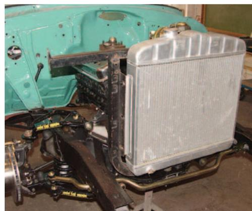
**Photo #2:** To mount an electric fan on the back side of the radiator, the radiator must be in the 6-cylinder position (in front of the core support). A 6-cylinder radiator and 6-cylinder core support may
