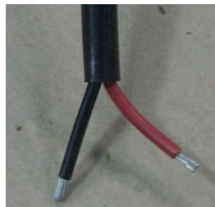
**Photo #10:** The electric fan has a black and red wire. If the fan is going to be used as a puller fan (behind the radiator) the BLACK wire would connect to a good ground and the RED wire would connect to an ignition-on 12-volt source. If the fan is going to be used as a pusher fan (in front of the core support) the RED wire would connect to a good ground and the BLACK wire would connect to the ignition-on 12-volt source. The fan can simply be wired to the ignition switch so the
