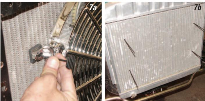
**Photos #7a & #7b:** Place the electric fan in the desired location and install the push pins through the fan mounting tabs and through the radiator core
