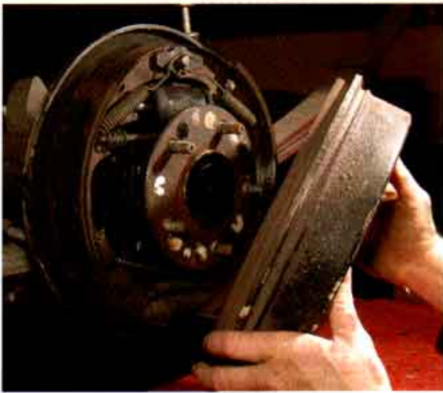
Photo #2: Remove the brake drums from the rear axle after backing off the adjustment on the brake shoes.
