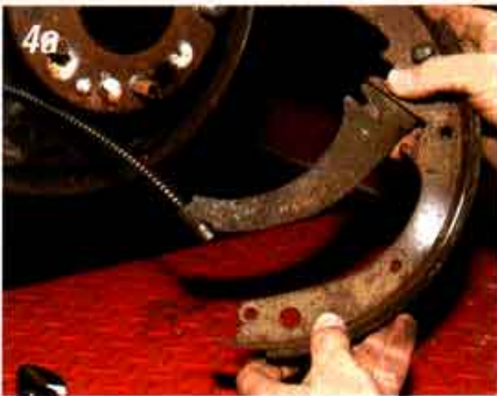
Photo #4a & 4b: The emergency brake cable attaches to the brake levers on the rear brake shoes. Disconnect the cable on both sides of the car. Use a pair of pliers or a screwdriver to depress the fingers on the ends of the cable sheath and remove the cable from the backing plates.
