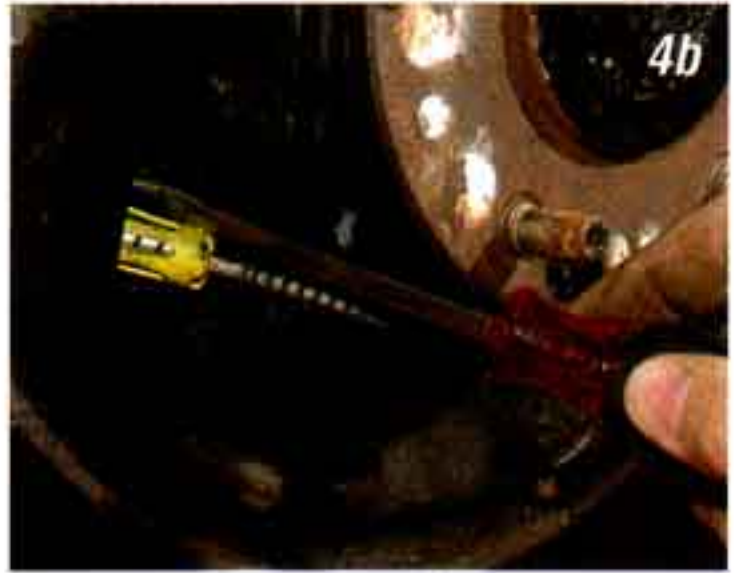
Photo #4a & 4b: The emergency brake cable attaches to the brake levers on the rear brake shoes. Disconnect the cable on both sides of the car. Use a pair of pliers or a screwdriver to depress the fingers on the ends of the cable sheath and remove the cable from the backing plates.
