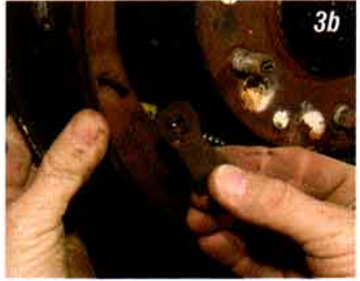
Photo #3a & 3b: Using a brake spring tool or a set of pliers, remove all the return and hold down springs from the brake shoes.
