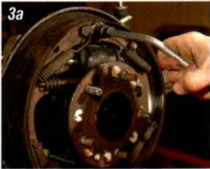
Photo #3a & 3b: Using a brake spring tool or a set of pliers, remove all the return and hold down springs from the brake shoes.
