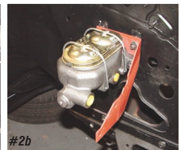
Photo #2a & 2b: When installing a non-power brake master cylinder, the upper two studs on the firewall are used to hold the GM style proportioning valve bracket. The lower two studs are used to hold the brake master cylinder in place.
