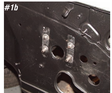
Photo #1a & 1b: The original master cylinder is held to the firewall with four 3/8" studs and nuts. The studs are mounted to the front of the brake pedal swing arm assembly and protrude through the four holes in the firewall.
