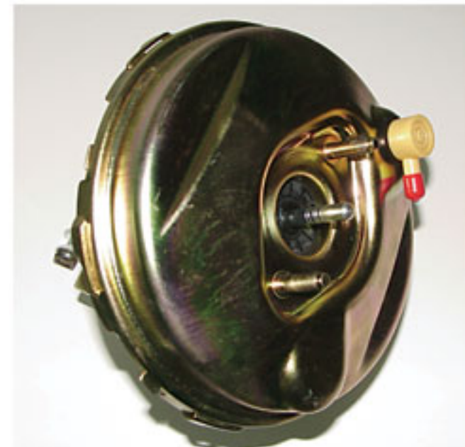
Photo #2: Not all 1968 to 72 A and F-body cars had the shallow dimple style master cylinder. Some applications used the master cylinder with the deep hole in the piston and required a booster with a long master cylinder pushrod.
