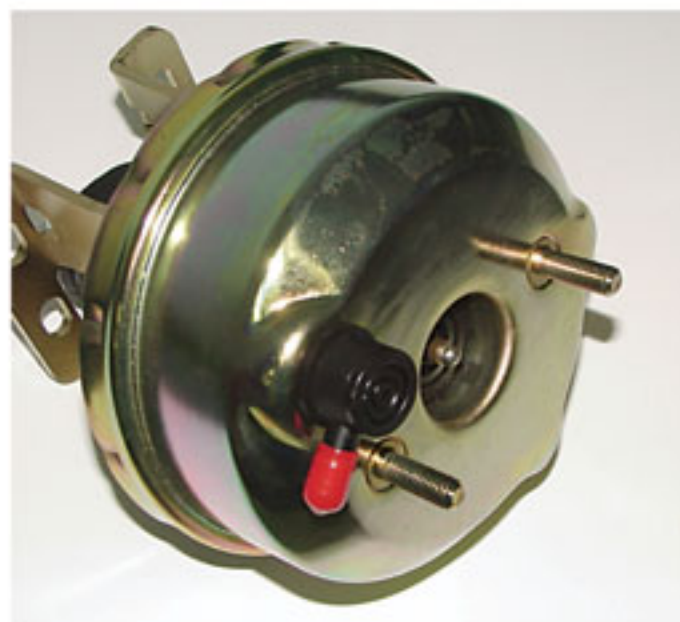
Photo #1: The aftermarket power brake boosters that are used in the Eckler's Classic & Late Great Chevy power brake/dual master conversions for the 1955 to 1964 cars accepts the common dual master cylinder from 1968 to 72 A and F-body cars. The aftermarket boosters have a
