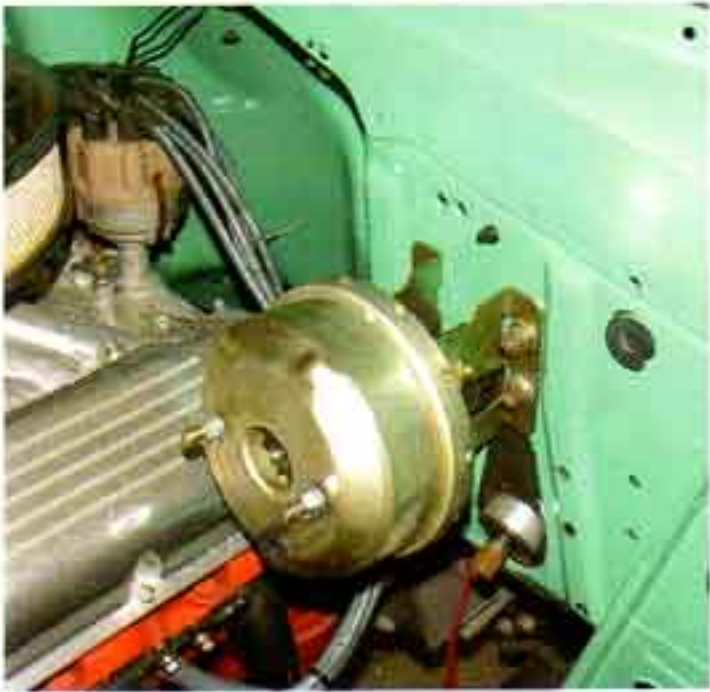
Photo #16a & 16b: Drill a 3/8" hole in the brake pedal swing-arm under the dash exactly 1" lower than the original clevis pin hole. The new power booster push rod will attach to this new hole to allow proper travel of the booster diaphragm.
