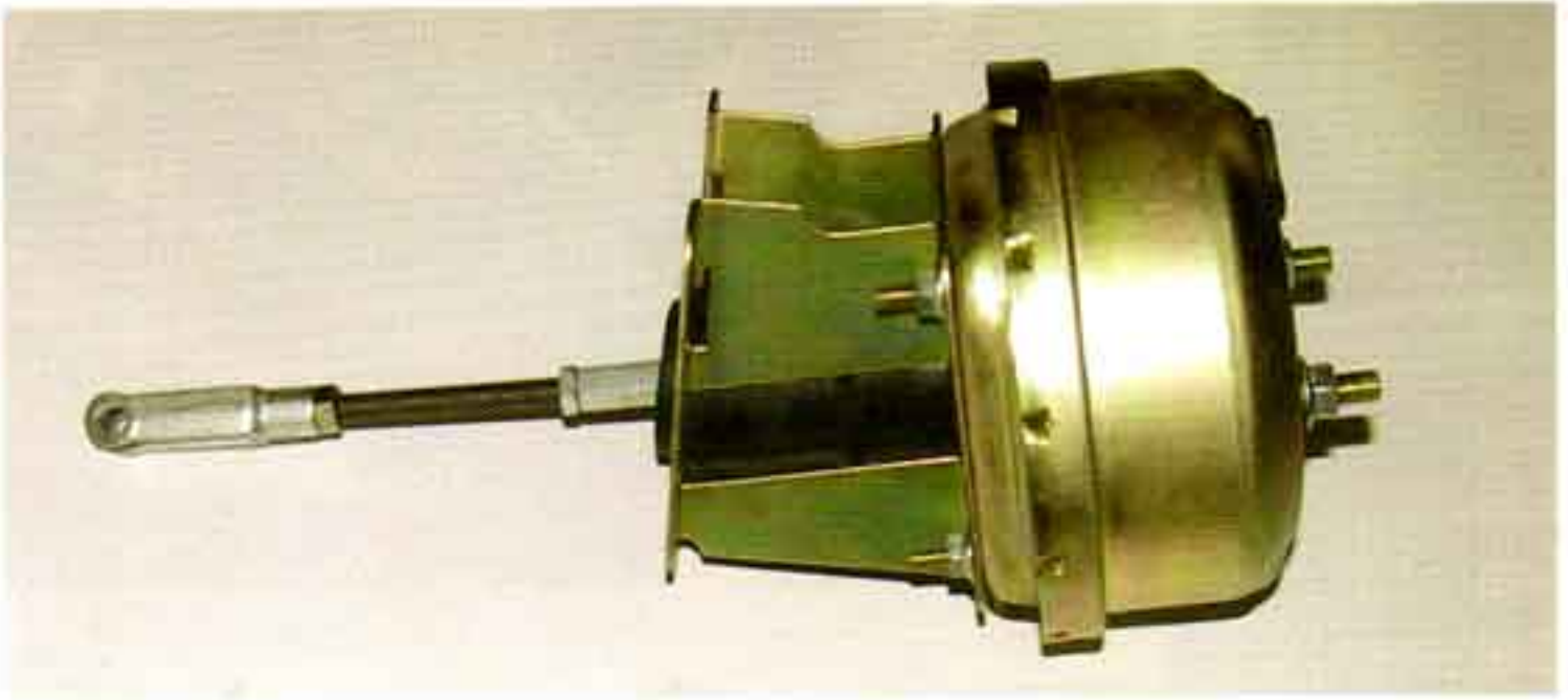
Photo #15: The 7" power booster will bolt directly to the firewall where the original brake master cylinder bolted on.
