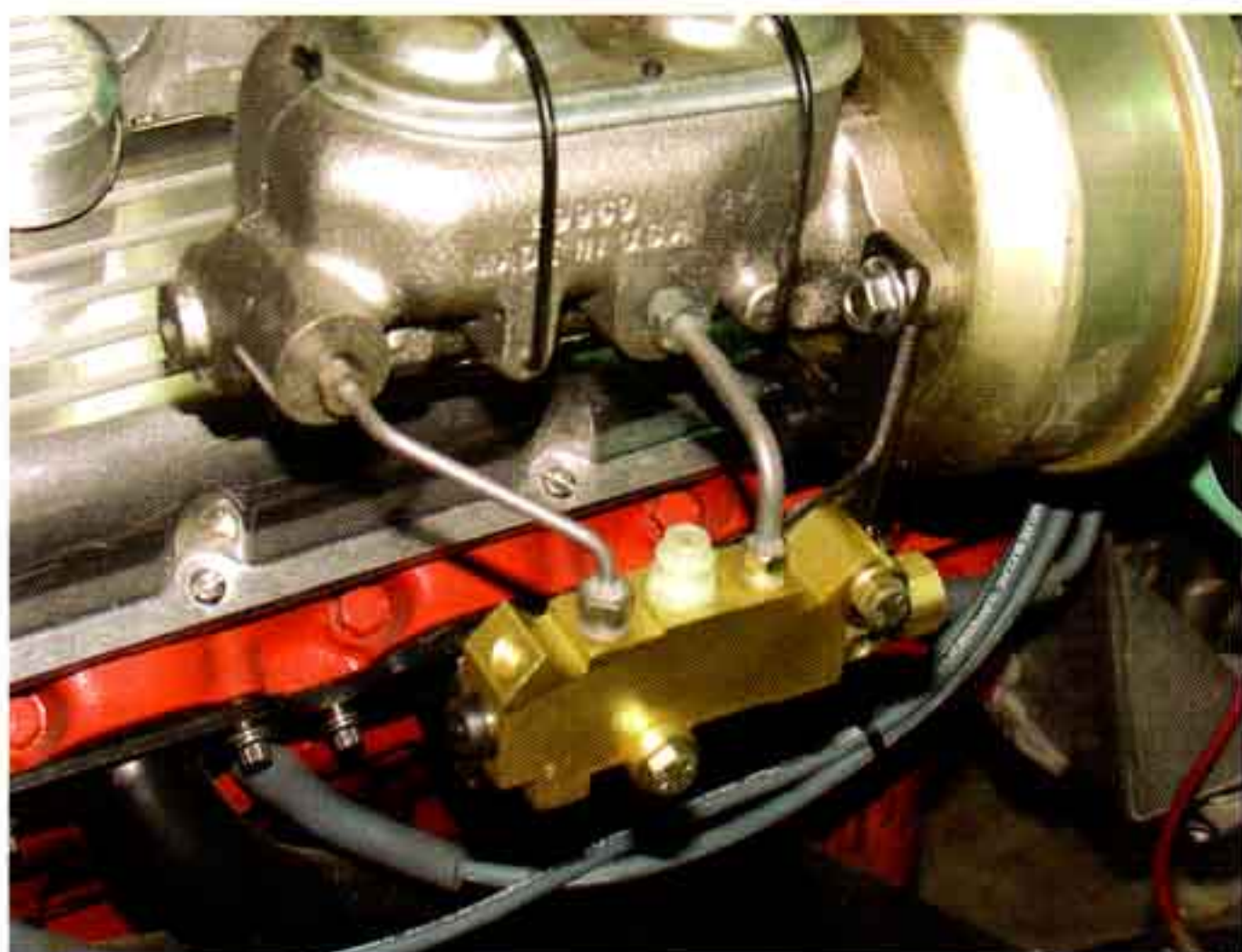
Photo #20: Install the pre-bent lines between the master cylinder ports and the proportioning valve.
