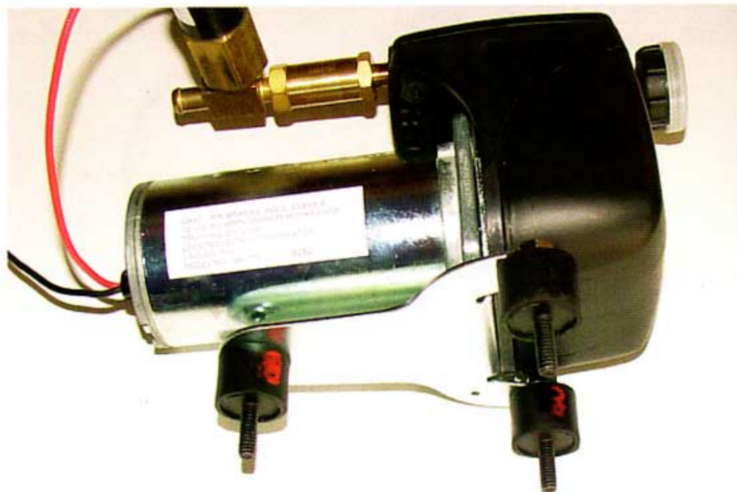
Photo #9: The vacuum pump may be mounted with three 1/4" studded insulators provided. This will keep the pump very quiet.
