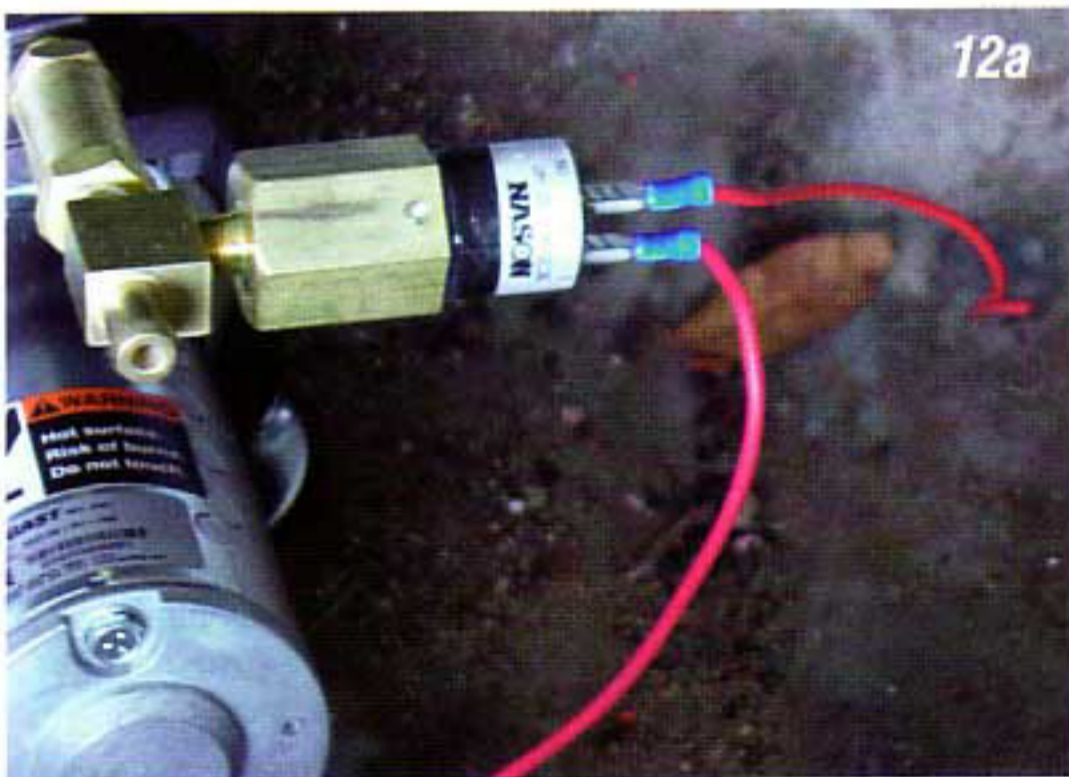
Photo #12a & 12b: Connect a power wire from the ignition switch to the other terminal on the pressure switch, this wire needs to be fused and only be hot when the key is on.
