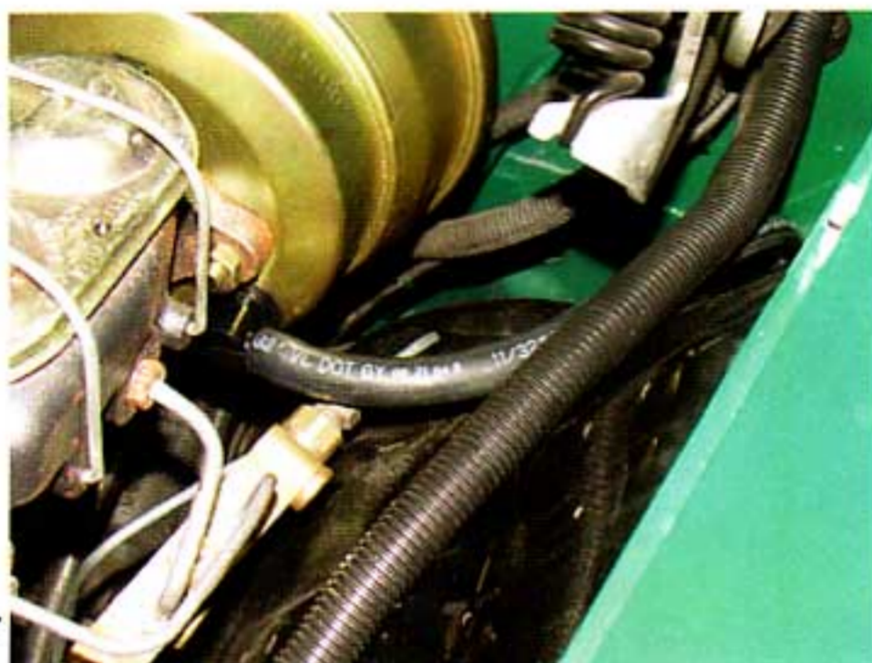
Photo #5: The vacuum pump can be mounted anywhere on the car. A clean, out of the way place to mount it is may be the trunk area. A 3/8" vacuum hose can be run to the rear of the car along the frame or under the carpet and sill area. Be sure to use a good quality hose so that the hose does not collapse or kink.
