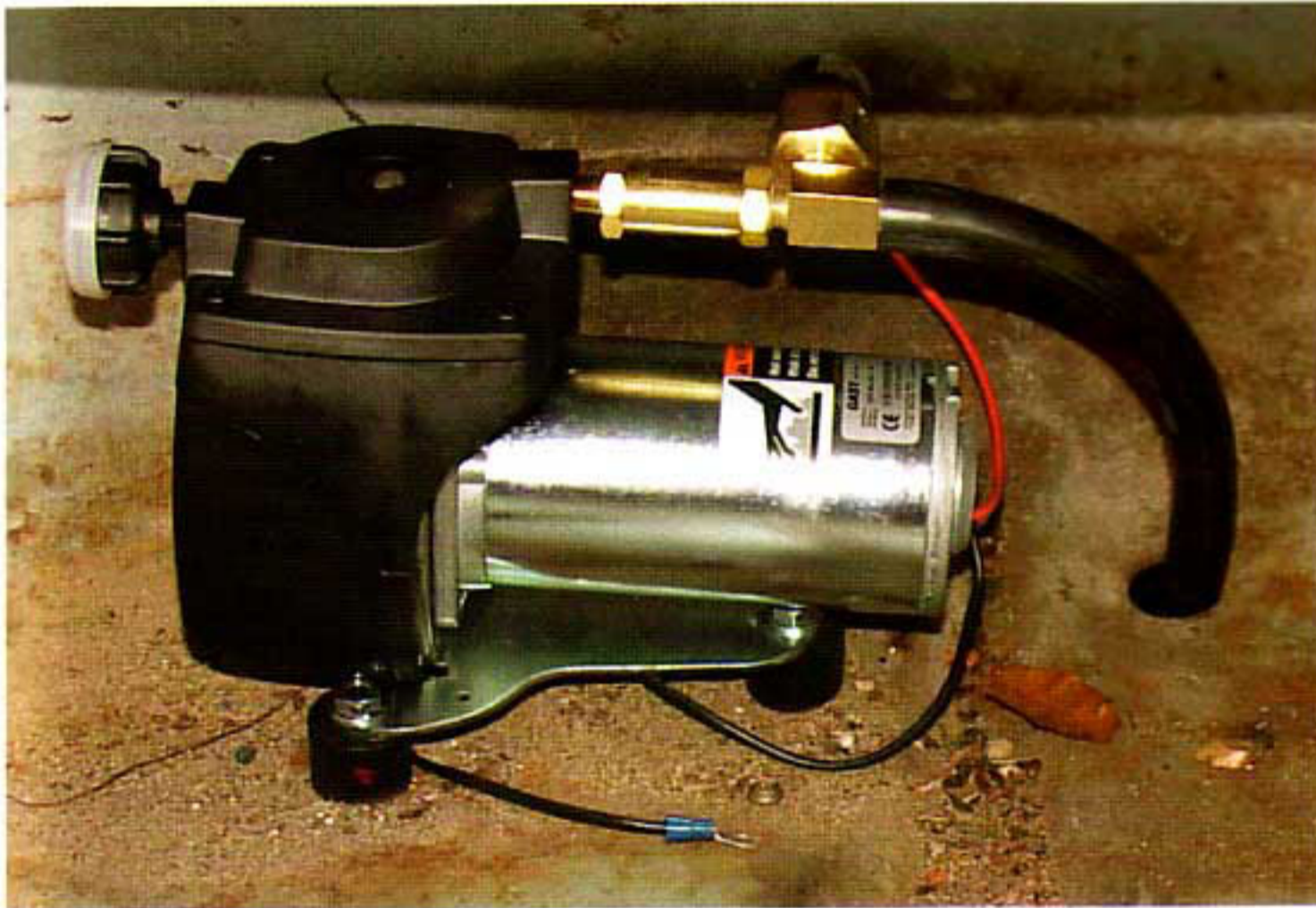
Photo #11: We removed one of the spare tire well plugs and fed the vacuum hose running from the booster up through the spare hole and connected it to the brass fitting on the vacuum pump.
