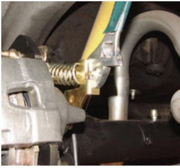
**Photo #11:** With the caliper installed over the rotor, the emergency brake eccentric in the caliper will need to be adjusted. Using an adjustable wrench, move the emergency brake lever on the caliper forward toward the front of the car five to ten times until the brake
