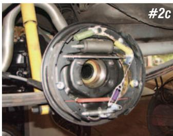
**Photo #2a & 2b & 2c:** The rear axles are held in the rear end housing with an outer retainer plate between the axle bearing and the axle flange, just like on an original 55-57 rear. Remove the four nuts behind the axle flange and using an axle puller or the drum with a couple of lug nuts on the wheel studs, pull the axle out of the rear end housing.
