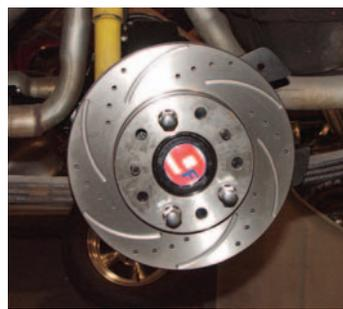
**Photo #9:** The brake rotors have the Chevy 5 on 4-3/4" bolt pattern and will fit the 7/16" wheel studs on the converted Ford axles. Using a couple of lug nuts, bolt the rotor into place. This will hold the rotor in place while installing the brake caliper.
