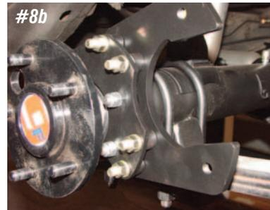
**Photo #8a & 8b:** The outer disc brake bracket bolts to the inner bracket with four 3/8" X 2" bolts. The outer bracket bolts to the inside of the inner bracket and has four spacers to properly align the caliper with the rotor. Torque these bolts to 35 ft/lbs.
