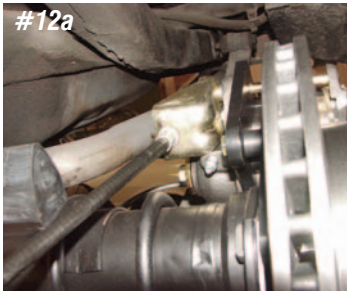
Photo #12a & 12b: A new one-piece rear emergency cable is supplied with the kit allowing the new rear disc brakes to be connected to the stock emergency brake adjuster under the car. The cable clips into the bracket on the caliper and the ball end of the cable hooks into the eccentric lever on the caliper.
