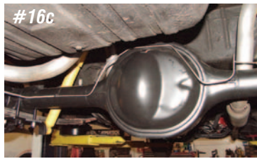
Photo #16a & 16b & 16c: The kit includes pre-bent brake lines that connect the calipers to the original brass junction block T on the rear end. The lines are bent to match up with the contour of the Ford rear and clip into the stock tabs on the rear end.
