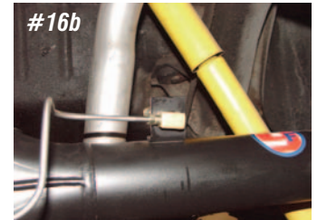
Photo #16a & 16b & 16c: The kit includes pre-bent brake lines that connect the calipers to the original brass junction block T on the rear end. The lines are bent to match up with the contour of the Ford rear and clip into the stock tabs on the rear end.
