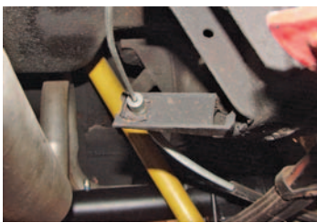
Photo #13: The new cable also connects to the original rear emergency brake cable bracket on the frame using clip P/N 34-114.
