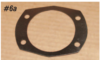
Photo #6a & 6b: A spacer is installed on the end of the axle housing to take the place of the brake backing plate. The original backing plate T-bolts can be used with the new disc brake brackets.
