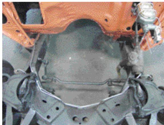
**Photo 8:** The new lines run across the back side of the front engine crossmember. Once our engine is installed the lines will be just about invisible! Good Luck. 🍀
