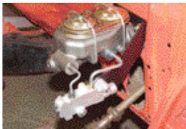
**Photo 5:** The new prebent brake lines connect to the proportioning valve and feed the left and right front wheels and also connect to the original brake line on the passenger side of the car for the rear brakes. The lines are all 3/16" in size for maximum brake pressure. They can be used with a stock steering box, a 605, 670 or Delphi power steering box or a rack and pinion system. They will clear side mounts or front mounts and small block or big block engines.
