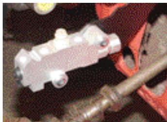
**Photo 3:** A proportioning valve must always be used when installing a dual master cylinder for the system to operate properly and provide the full safety features of the dual system. Our P/N 20-32 or 20-32C is a GM style 5-port
