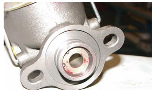
**Photo #3:** A non-power brake master cylinder for drum or disc brakes will have a deep hole in the rear of the piston for the brake pedal push rod. A power brake master cylinder will have a shallow dimple in the piston for the brake booster push rod.
