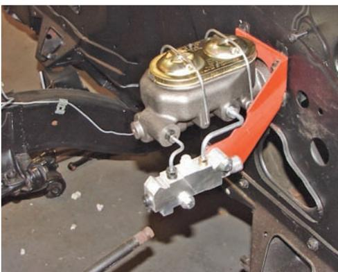
**Photo #7:** With the lines still loose, push on the proportioning valve flexing the brake lines until the holes in the valve line up with the holes in the mounting bracket and there
