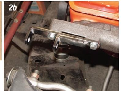
**Photos 2a & 2b:** The alternator bracket **P/N 207-68** is similar to many universal style chrome brackets that you can purchase, but ours has a different bolt pattern to match up to the exhaust manifold. It also has a different offset to allow the alternator to line up with the pulleys on a short water pump. The bracket and pulley kit **#18-290** includes two 3/8" X 3/4" bolts and lock washers to hold the alternator mounting bracket to the manifold.
