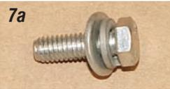
**Photos 7a & 7b:** The adjusting arm attaches to the alternator adjusting ear on the alternator with a supplied 5/16" X 1" bolt with flat washer and lock washer.
