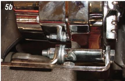
**Photos 5a & 5b:** The bracket and pulley kit #18-290 includes a 3/8" X 3" bolt, lock nut and five flat washers to be used for proper shimming. Our installation required three washers on the back side of the alternator mounting ear to give us proper pulley and belt alignment.
