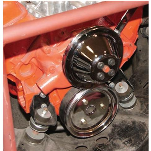
needed. The water pump pulley is held to the water pump with four supplied 5/16" X 3/4" fine thread bolts and flat washers. The crankshaft pulley is held to the harmonic balancer with three supplied 3/8" X 3/4" fine thread bolts and lock washers.
