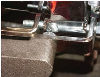
**Photo 4:** The mounting ear on the alternator is about 1/2" narrower than the mounting legs on the bracket. This will allow for front to rear adjustments when lining up the pulleys.
