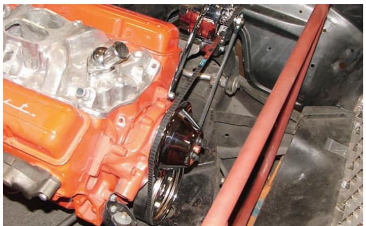
**Photo 9:** Last, install the fan belt. With the correct matching pulleys and the alternator positioned correctly the belt will line up perfectly and upgrade your car to a modern charging system! Good Luck!
