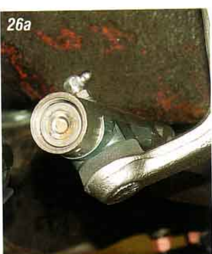
Photo #26a & 26b: Next screw the end cap in flush with the end of the drag link. This will put the proper preload on the springs, seats and spacers. Now install a new cotter pin through the hole in the end of the drag link to keep the end cap in place.
