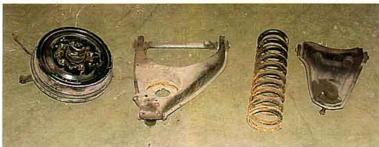
Photo #8: With everything removed, we can now start the restoration. Make sure to keep track of/mark the left and right side parts as they are different.
