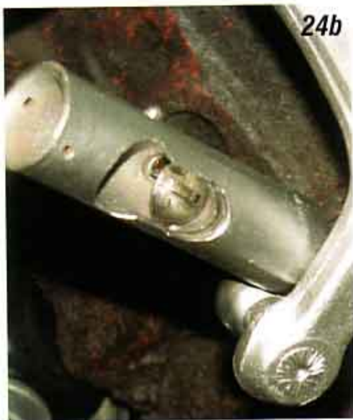
Photo #24a & 24b: The driver's side of the drag link attaches to the ball on the pitman arm. There are two seats, two springs and two spacers on each side of the ball that will hold the drag link to the pitman arm. If the ball seats are worn and in need of replacement, they may be replaced with new ones included in kit, P/N 21-64.
