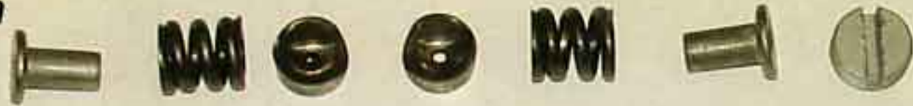
Photo #24a & 24b: The driver's side of the drag link attaches to the ball on the pitman arm. There are two seats, two springs and two spacers on each side of the ball that will hold the drag link to the pitman arm. If the ball seats are worn and in need of replacement, they may be replaced with new ones included in kit, P/N 21-64.
