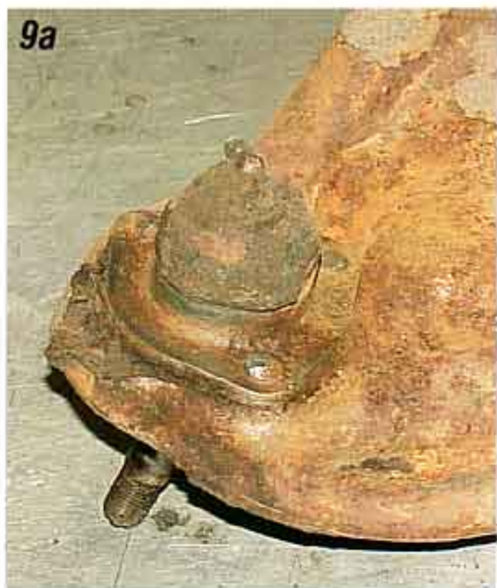
Photo #9a & 9b: The upper and lower ball joints were riveted to the control arms from the factory. Using a grinder or chisel, remove the head of each rivet. The remains of the rivet can be driven out of the control arm using a hammer and punch.
