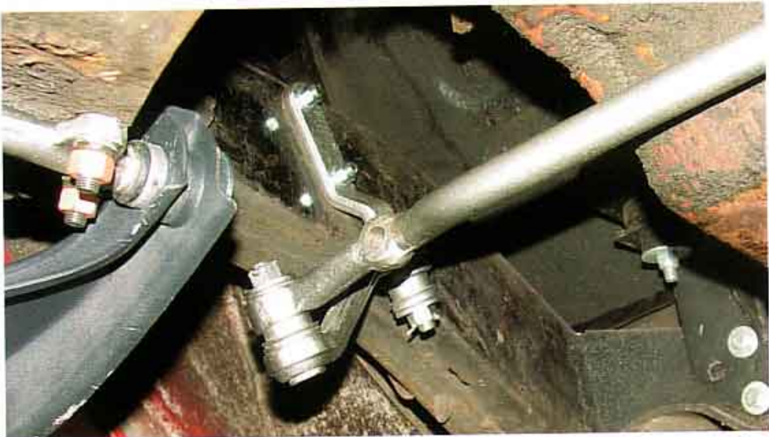
Photo #23: The idler arm bolts to the passenger side frame with two 3/8" carriage bolts and nuts, P/N 34-170. Attach the bushing end of the drag link to the idler arm with the original nut and a new cotter pin.
