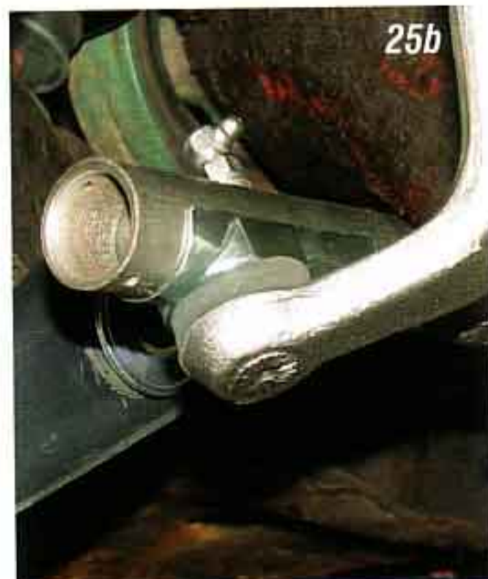
Photo #25a & 25b: There is a dust seal and metal shield, P/N 53-56, that fits over the end of the drag link to keep dirt and moisture out of the drag link. With the dust seal and shield in place install the end of the drag link onto the pitman arm ball.
