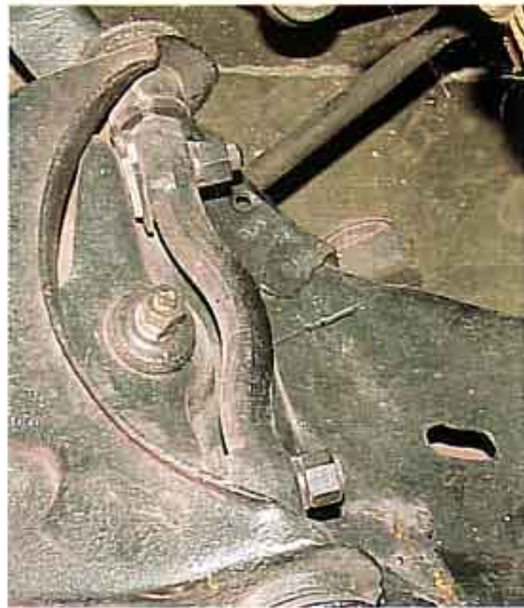
Photo #7: The upper control arm is held to the frame with two 7/16" studs and special nuts. The lower control arms are held to the bottom of the frame with four 7/16" bolts, lock washers and nuts. Remove all hardware and remove the upper and lower control arms.
