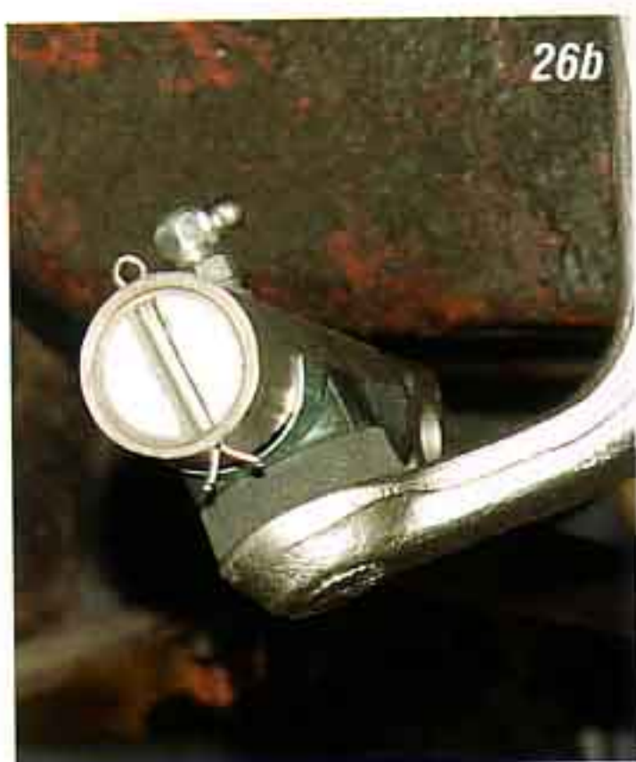
Photo #26a & 26b: Next screw the end cap in flush with the end of the drag link. This will put the proper preload on the springs, seats and spacers. Now install a new cotter pin through the hole in the end of the drag link to keep the end cap in place.
