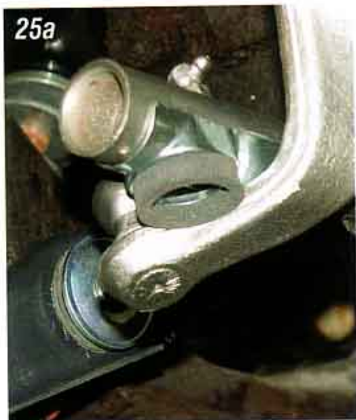
Photo #25a & 25b: There is a dust seal and metal shield, P/N 53-56, that fits over the end of the drag link to keep dirt and moisture out of the drag link. With the dust seal and shield in place install the end of the drag link onto the pitman arm ball.
