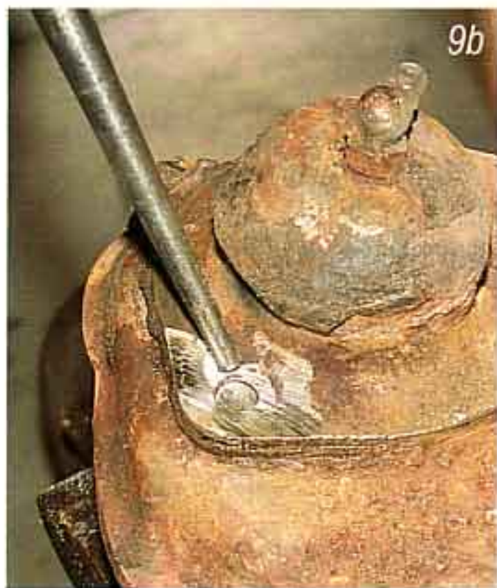
Photo #9a & 9b: The upper and lower ball joints were riveted to the control arms from the factory. Using a grinder or chisel, remove the head of each rivet. The remains of the rivet can be driven out of the control arm using a hammer and punch.
