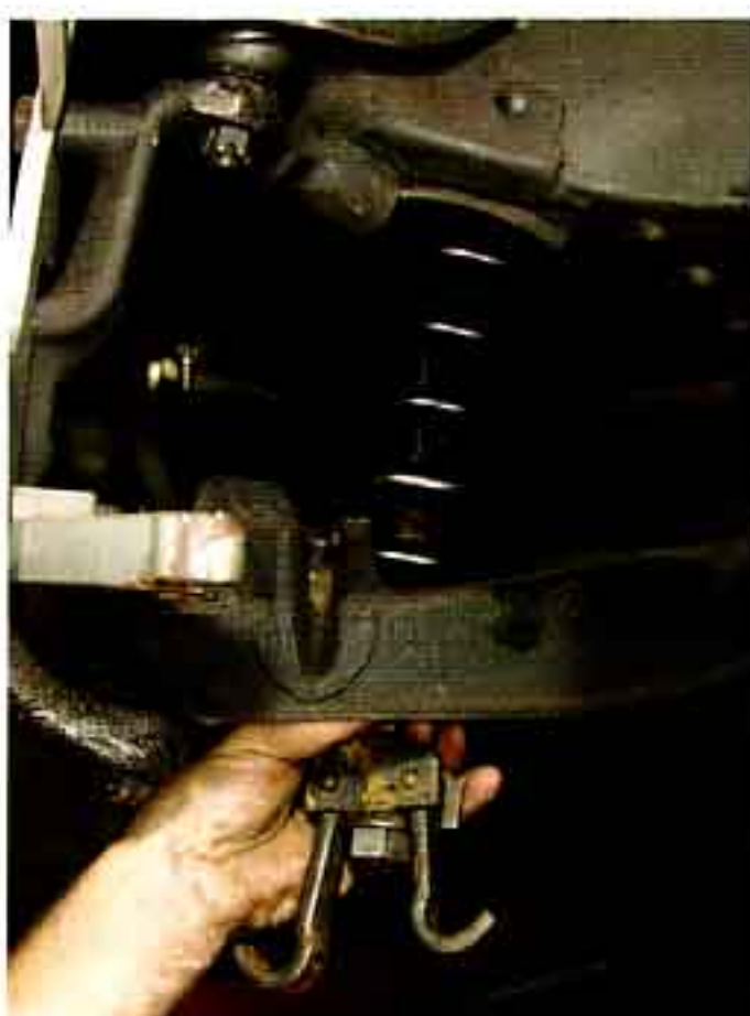
Photos #9, #10a & #10b: A coil spring compressor must be used to install the new coil springs. Place the coil spring in the lower control arm pocket. Raise the control arm and spindle assembly up to align with the upper ball joint and reinstall the upper ball joint nut. Remove the coil spring compressor.
