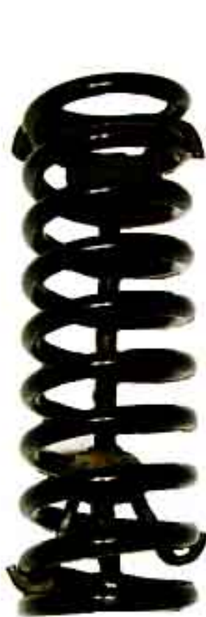
Photos #9, #10a & #10b: A coil spring compressor must be used to install the new coil springs. Place the coil spring in the lower control arm pocket. Raise the control arm and spindle assembly up to align with the upper ball joint and reinstall the upper ball joint nut. Remove the coil spring compressor.
