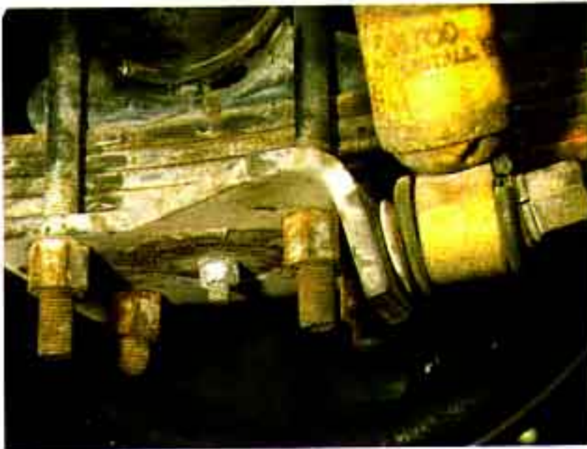
Photo #17: The rear end is held to the leaf springs with two U-bolts, nuts and a lower shock plate per side. First remove the 3/4" nut that holds the shock to the lower shock plate.
