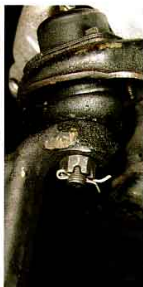
Photos #9, #10a & #10b: A coil spring compressor must be used to install the new coil springs. Place the coil spring in the lower control arm pocket. Raise the control arm and spindle assembly up to align with the upper ball joint and reinstall the upper ball joint nut. Remove the coil spring compressor.
