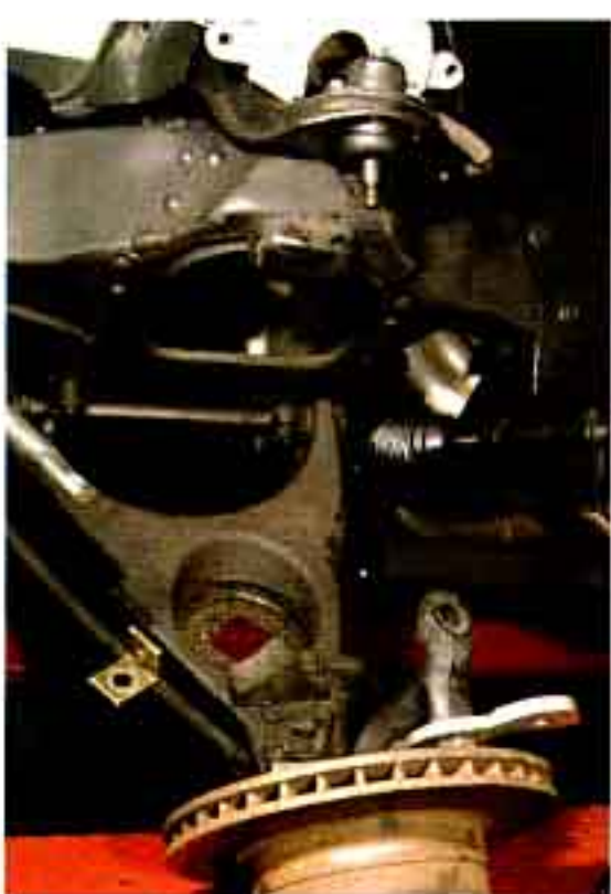
Photo #7: The lower control arm, coil spring and spindle will swing down, allowing the coil spring to be removed.
