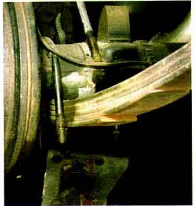
Photos #18a & #18b: Remove the four 3/4" nuts from the U-bolts and remove the lower shock plate.
