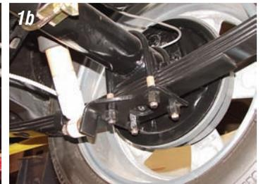
**Photos 1a & 1b:** The front of the rear leaf springs are held to the frame with a bracket or "perch" that is welded to the outboard side of the frame rails. The rear end housing is held to the leaf springs with two 1/2" U-bolts, four tall nuts and a lower shock plate on each side.
