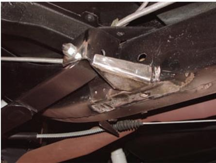
**Photo 5:** The front traction bar bracket is welded to the frame beneath the front factory leaf spring bracket. The frame must be cleaned of any paint, dirt or rust before welding the bracket in place.
