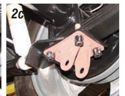
**Photos 2a, 2b & 2c:** The left and right rear traction bar brackets are the same and mount to the bottom of the stock rear lower shock plates. The brackets are held in place using the existing four U-bolt nuts. With the rear traction bar brackets installed, torque the four nuts to 65 ft/lbs. If the threads on the U-bolts do not protrude through the heads of the four nuts, replace the U-bolts with longer ones P/N 21-33.
