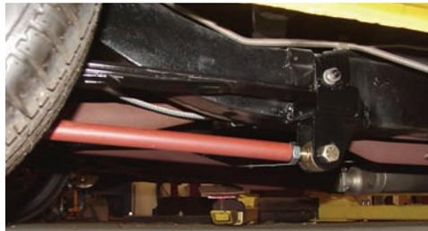
**Photo 9:** Now, set the car on the ground and install the left and right traction bars using the supplied 3/4" bolts and lock nuts. Torque the
