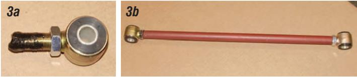
**Photos 3a & 3b:** Each traction bar has one left hand and one right hand threaded rod end with jam nuts. With the threaded rod ends on each end of the bar, the preload of the traction bar can be adjusted without removing the traction bar like other brands. Before threading the rod ends in, lubricate the threads with anti-seize or a good quality grease.
