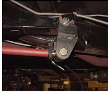
**Photo 7:** Connect the rear of the traction bar to the rear bracket at the lower shock plate with the supplied 3/4" X 2" bolt and locking nut leaving the nuts loose at this time. Now raise the front mounting bracket into place and tack weld the bracket to the frame.
