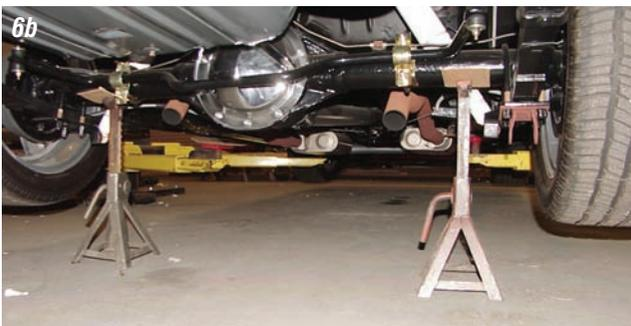
**Photos 6a & 6b:** The rear suspension must be in the ride height position when the front bracket is welded to the frame.
