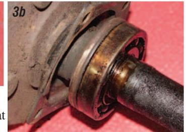
**Photos 3a & 3b:** The axle bearing cover has four studs that hold the axle to the rear end housing. These must be removed to allow the bearing to be pressed off. Using a hammer, tap the studs out of the bearing cover.
