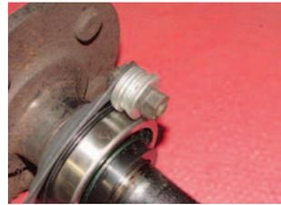
**Photo 8:** To install the axle retaining plate studs, simply stack up about seven or eight washers on the stud and using the backing plate nuts pull the studs into place.
