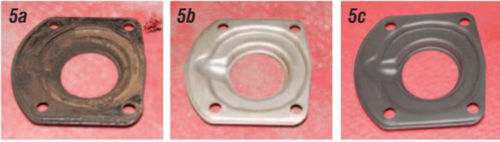
**Photos 5a, 5b & 5c:** The axle bearing cover has a gasket P/N 03-32 or 563206 that keeps the brake dust away from the axle bearing. These gaskets should always be replaced. We cleaned our bearing cover and painted it chassis black.
