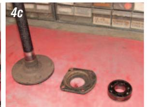
**Photos 4a, 4b & 4c:** A hydraulic press must be used to remove the axle bearing. Before applying any pressure to the bearing, wrap a heavy towel or rag over the bearing. If the bearing breaks while being pressed off, the towel will retain any broken pieces and help prevent any injury to you.
